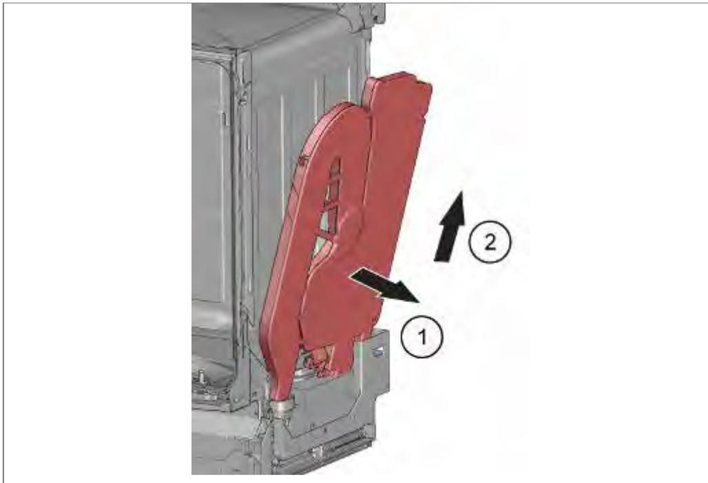
1. Tilt the fleet reservoir / duct away from the device
