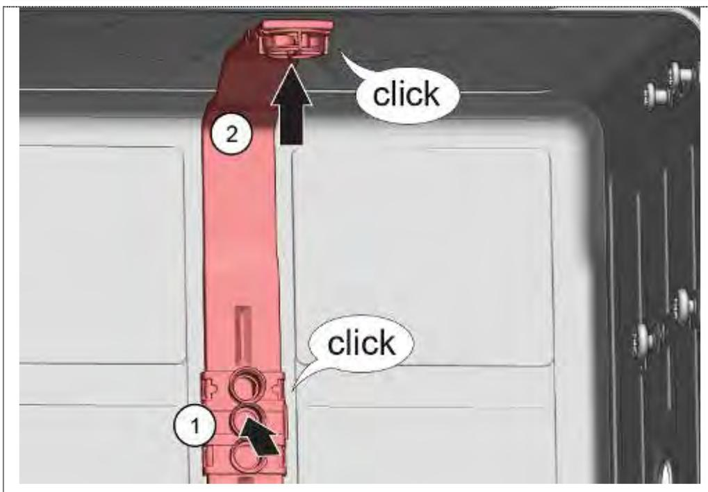
1. Lock the feeding pipe engage into the coupling site.
