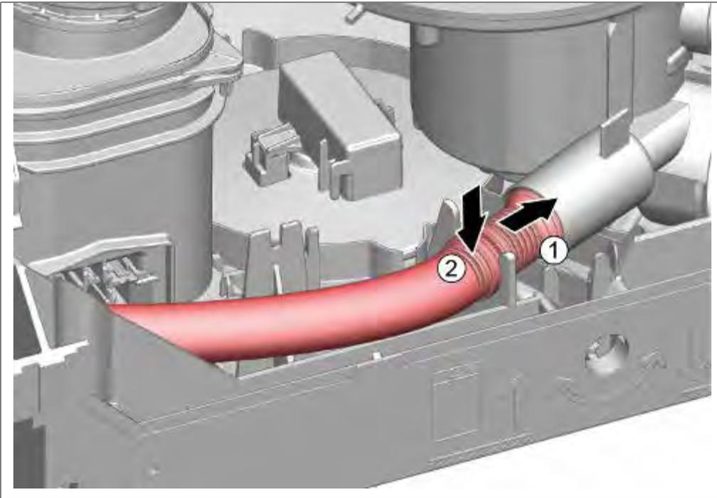
1. Push drainage hose into the pump sump.
