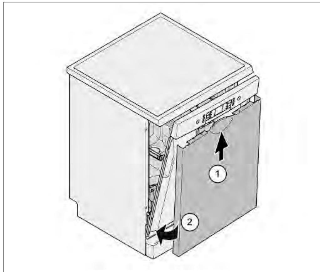
1. Push outer door with the upperside at an angle under the fascia.
