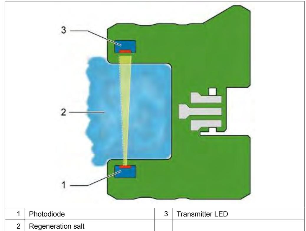
The salt level is detected via a light barrier. If the regeneration salt runs low, the line in the light barrier is freed and the electronics detect "Add salt".
