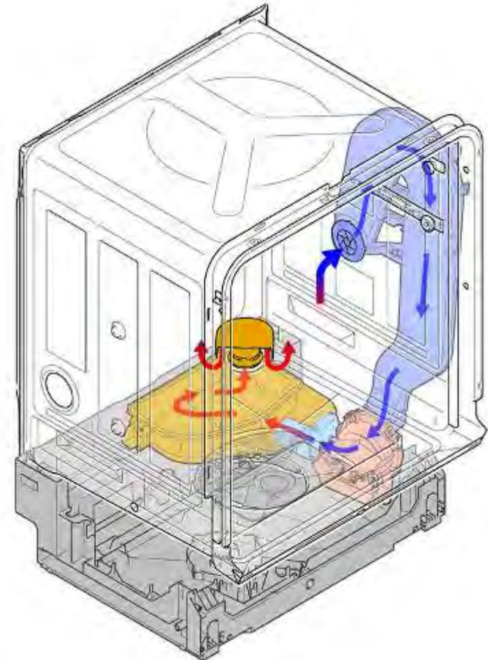
Airflow in the zeolithsystem
