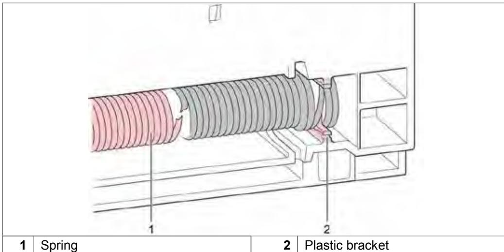
Spring system installed in reverse order. Fasten spring in the holder provided base carrier.
