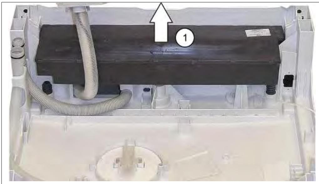
1. Remove the weight upwards.
