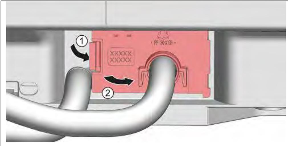
1. Loosen the panel catch mechanism.
