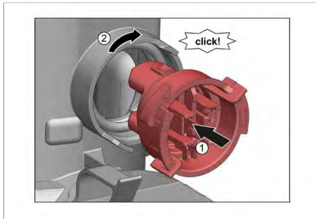
1. Press Aquasensor with board edgewise into the pump sump.
