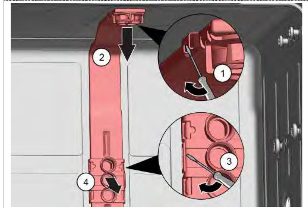
1. Loosen the upper catches on the optional sprinkler disc carefully.
