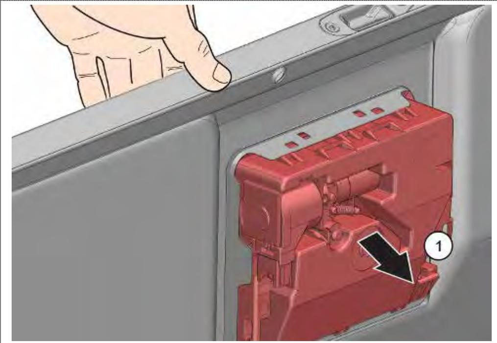
1. Engage dispenser evenly in the door and ensure that all 8 catch mechanisms have engaged.
