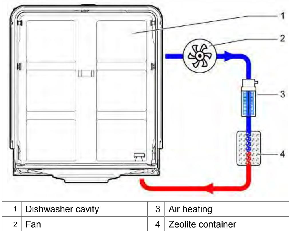
The dishes are heated up to 35°/45°C following rinsing with rinse-aid.. The interior now contains warm moist air.
