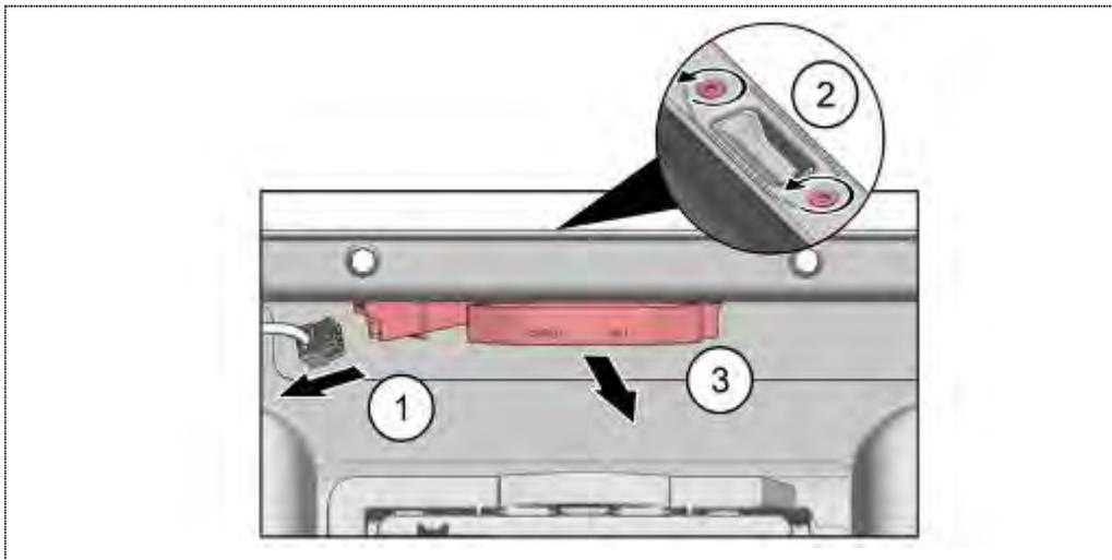
1. Carefully remove electrical connections (1).
