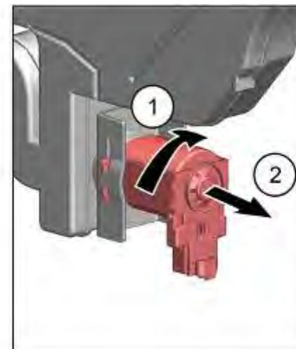
1. Remove the drainage valve by rotating it in a clockwise direction.
