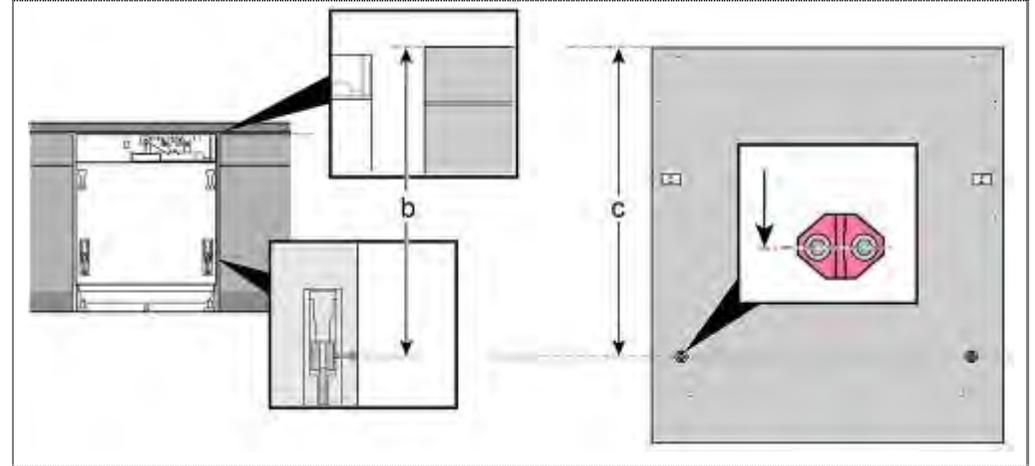
The distance **(b)** from the upper edge of the neighbouring front to the clamping screw of the glider must correspond to the distance **(c)** from the upper edge of the furniture sheet up to the middle of the connection clip.
