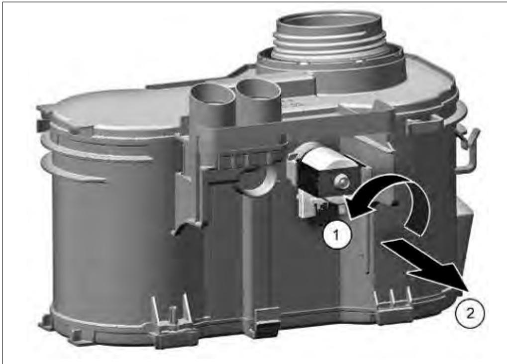
1. Rotate valve anti-clockwise.
