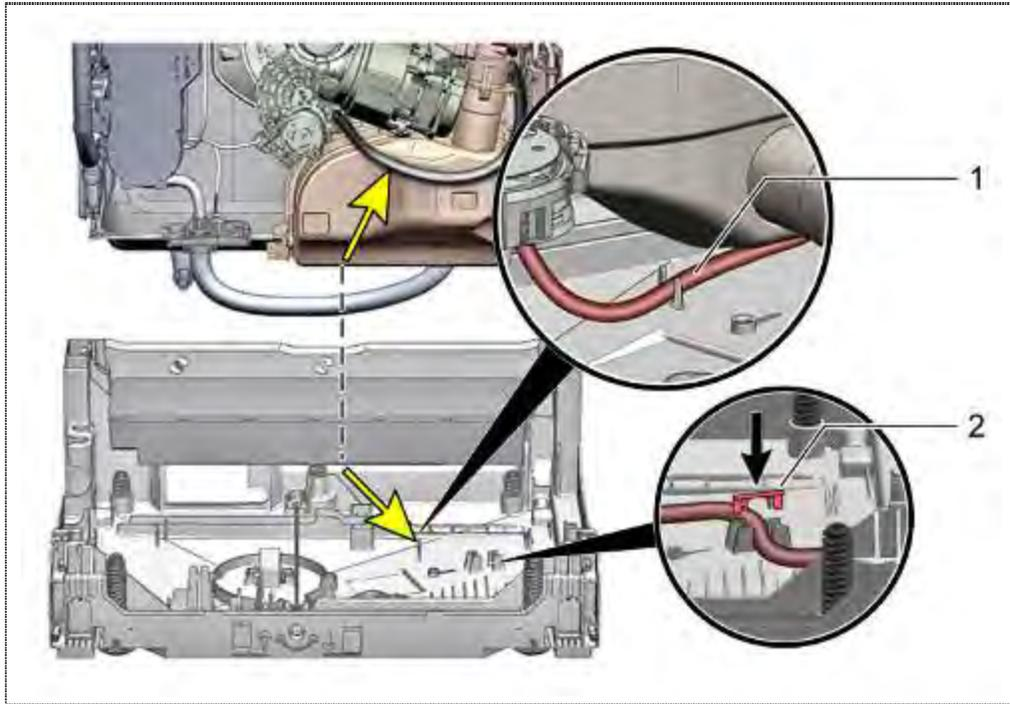
1. Insert the tube of the optional water storage tank in the provided holder.
