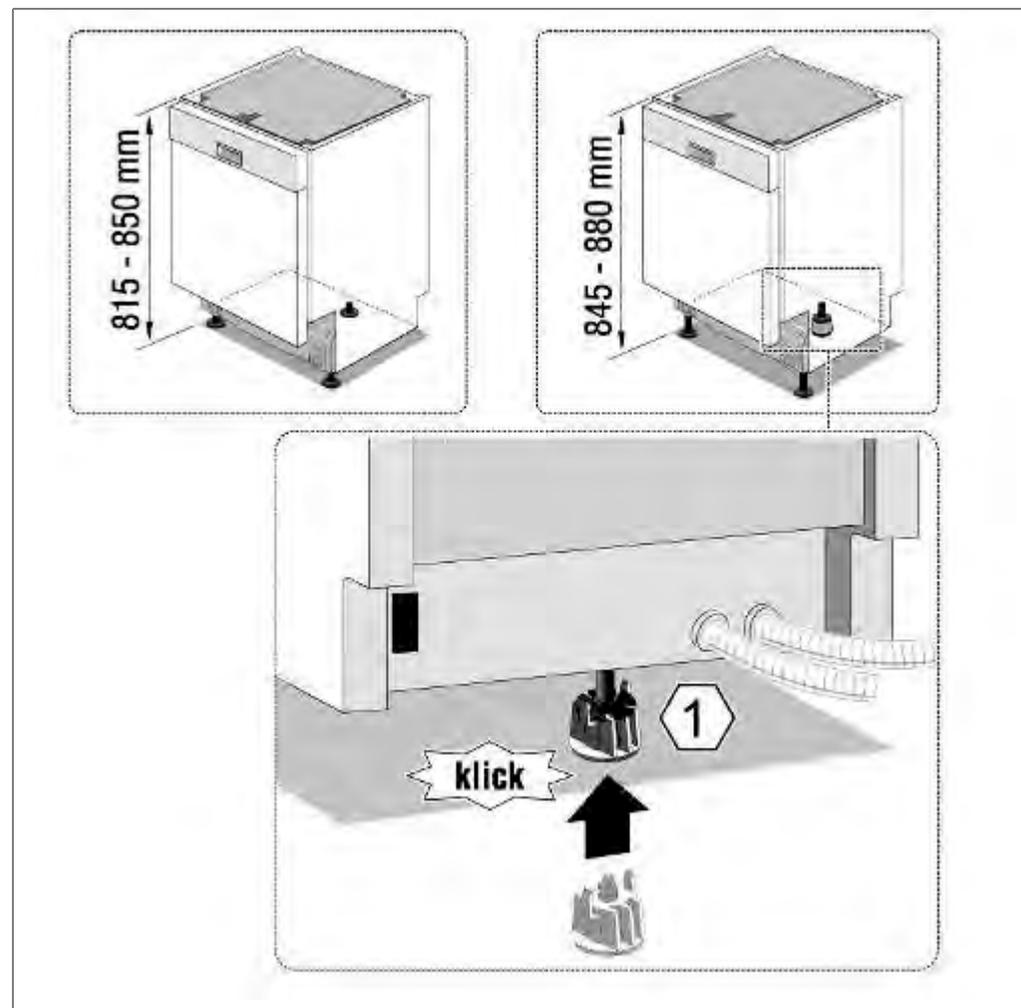
Illustration 2: Built-in & built-under appliance with adaptor 1
