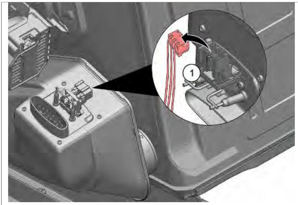
1. Disconnect electrical connections on the zeolite container.
