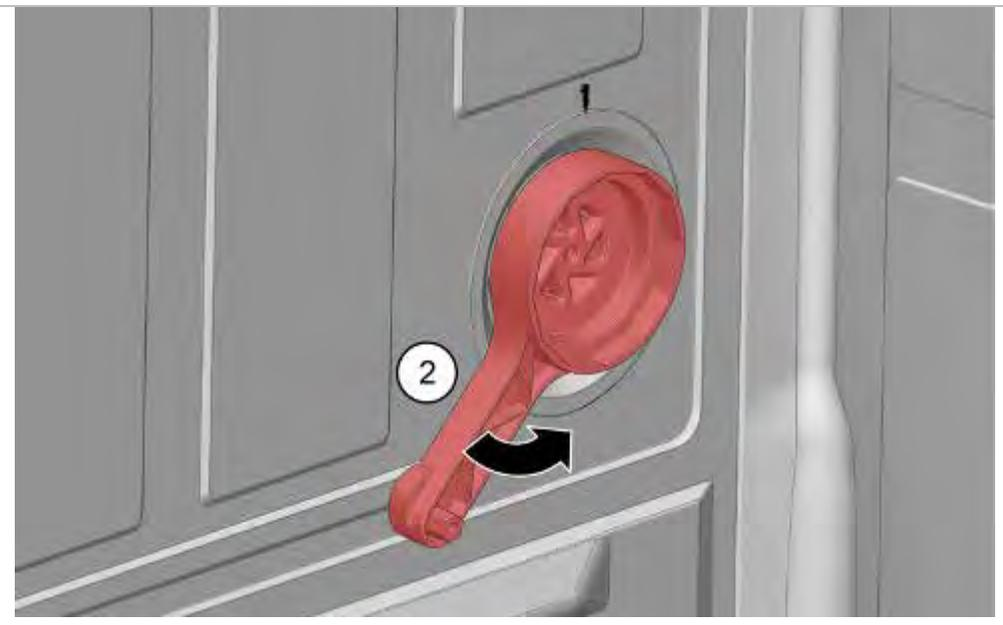
1. Remove the expansion opening nut with special tool.
