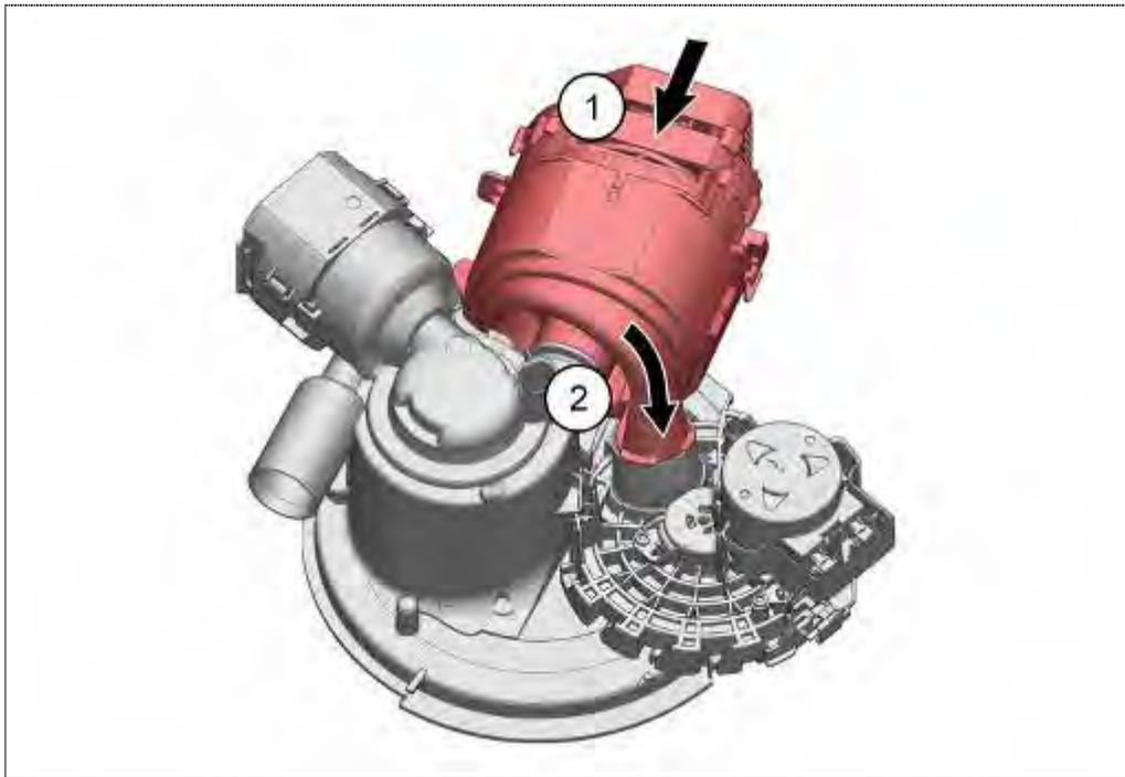
1. Push heating pump onto the pump sump and
