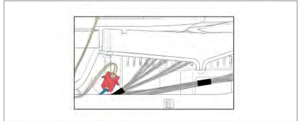
Disconnect the electrical connection to the power module.
