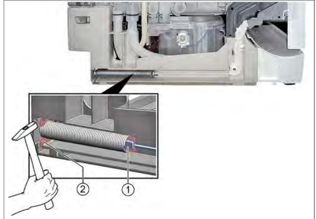
Connect rope to the spring (1) and hammer metal retaining plate into designated groove in base group (2)
