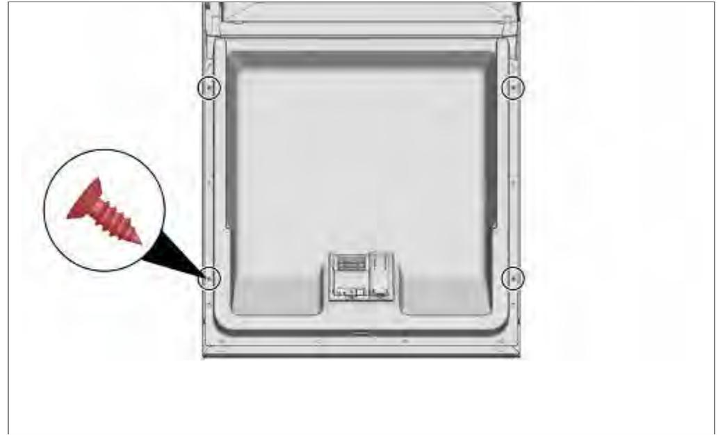
1. Remove the 2 screws on each side of the inner door.
