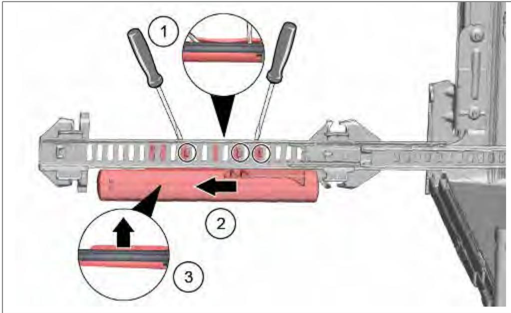
1. With a small screwdriver, carefully separate the latches from the glide.
