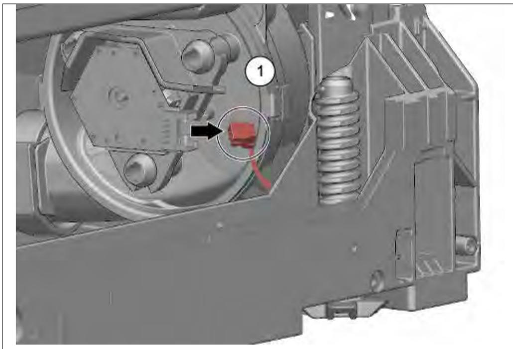
1. Disconnect electrical connection on the fan motor.
