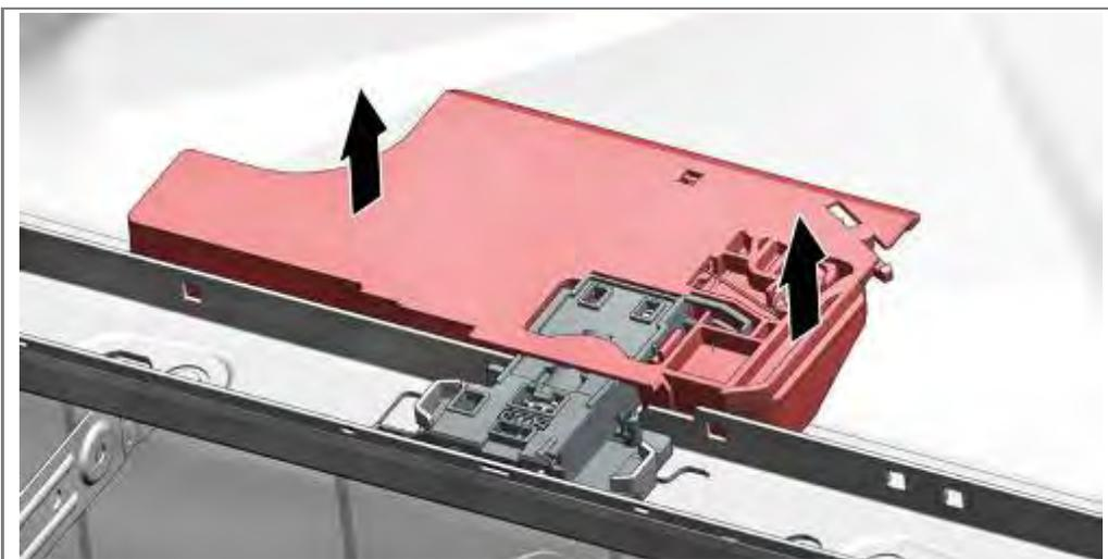
1. Remove the door opening module by lifting straight up.
