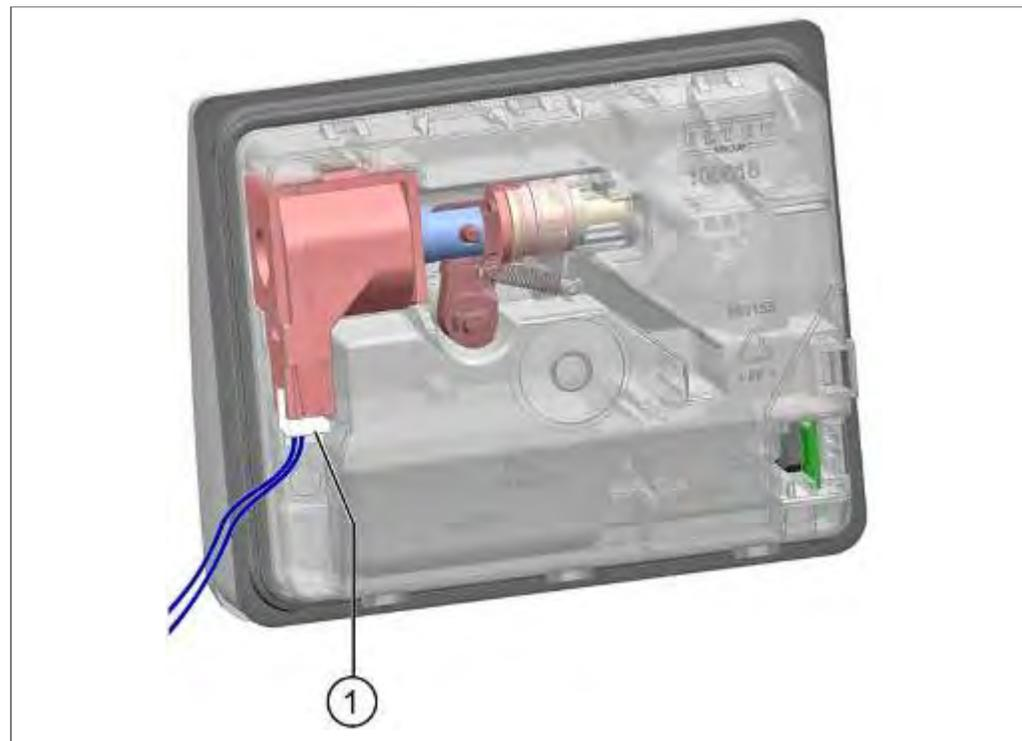
1. Disconnect plug-and-socket connection.
