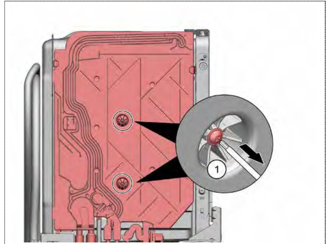
1. Remove both Torx screws on the outside of the tank
