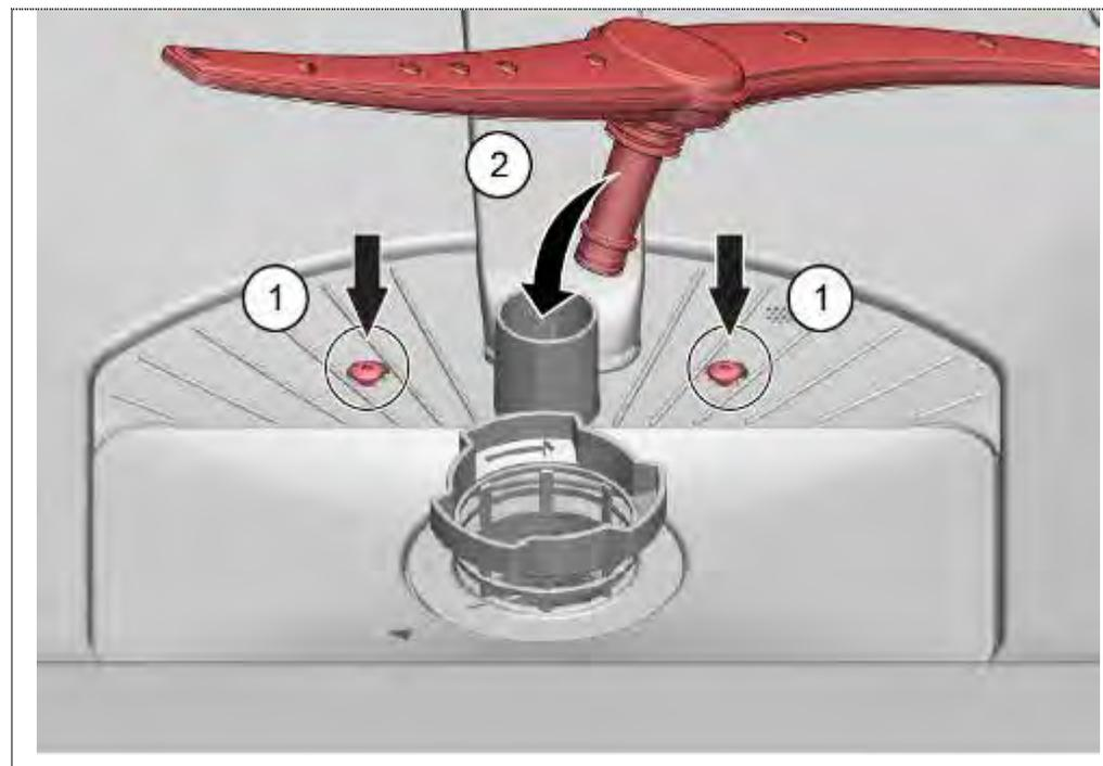
1. Screw both Torx screws to the pump sump.
