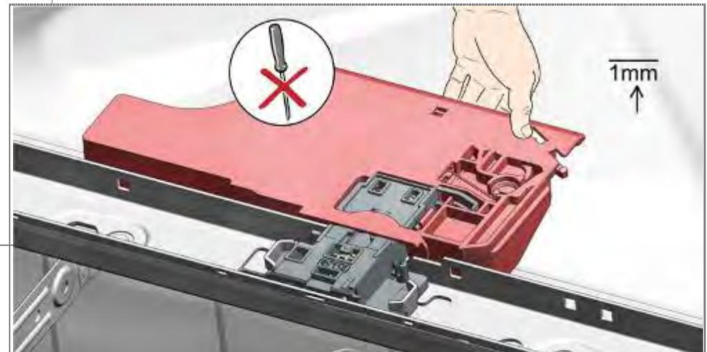
1. The module may have become attached to the bitumen in which case it needs to be separated.
