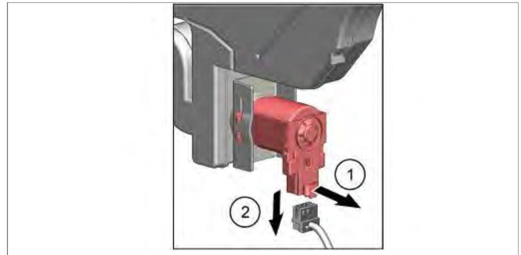
1. Disconnect plug-and-socket connection and measure the resistance.
