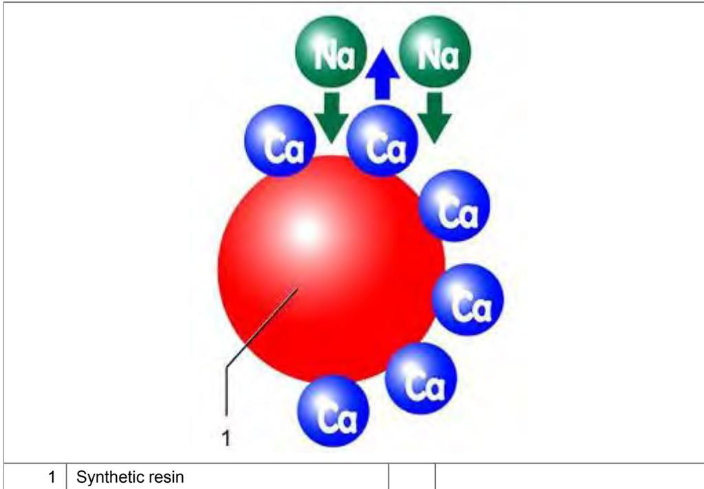
To make the ion exchanger functional again, a concentrated salt solution (sodium chloride) is conveyed from the salt dispenser by the water softener. Due to the large surplus the sodium ions from the salt solution displace the calcium and magnesium ions and attach themselves to the exchange compound. The ion exchanger is now “loaded” (regenerated) again and ready for use.
