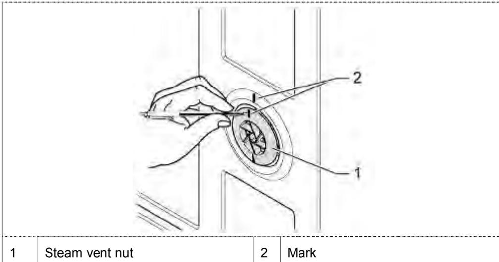
1. Mark the steam vent nut in mounting position.
