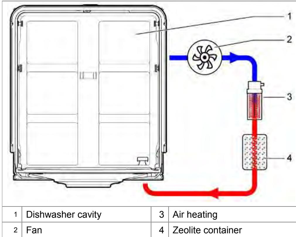
The zeolite must be dried before the system can absorb moisture once again. This takes place during the cleaning phase.
