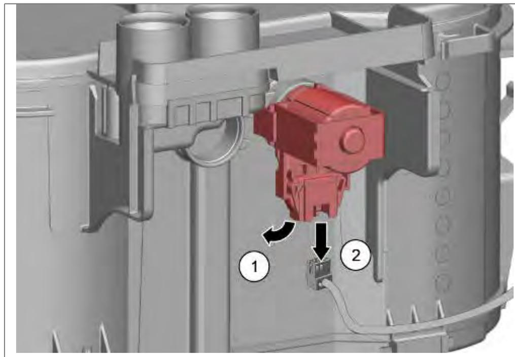
1. Loosen plug-and-socket connection on the regeneration valve.
