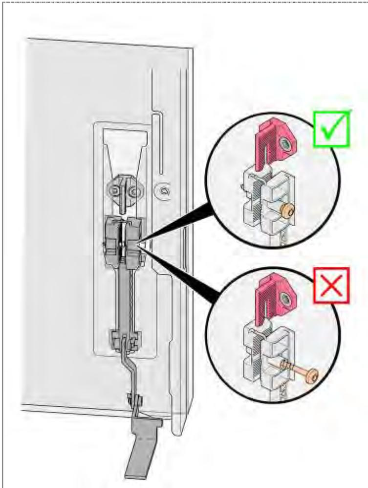
The screw must be screwed in, but not fixed.
