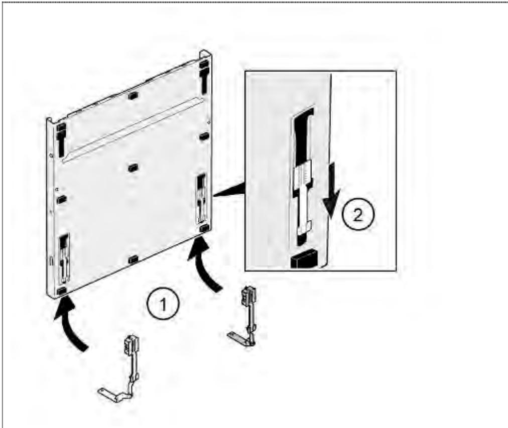
1. Insert both slideelements to the conduct
