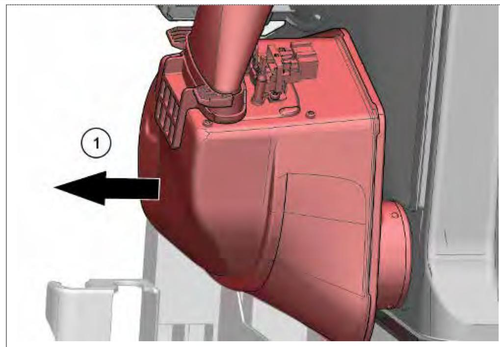
1. Remove Zeolit container from tub.
