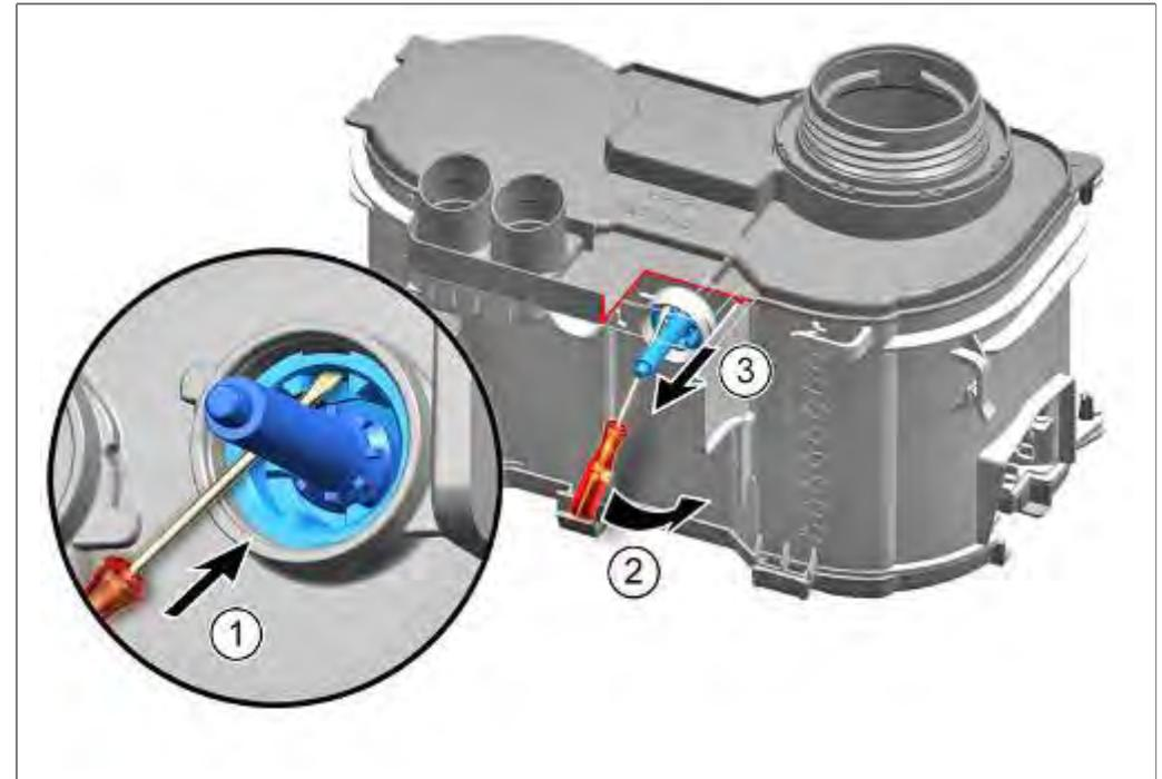
1. Insert a small screwdriver in the valve position
