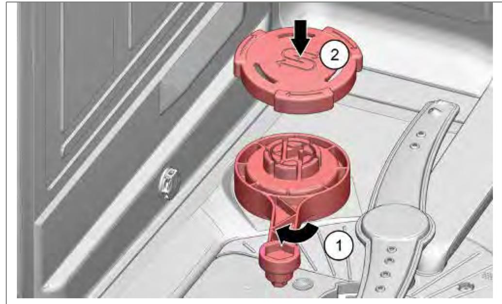
Push water softening system from below into the rinsing tank.
