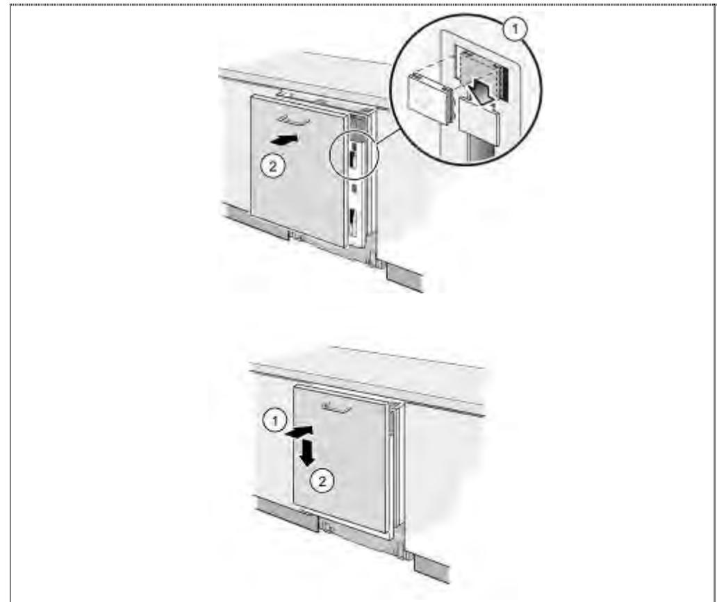
1. Insert sliding elements correctly into the guides.
