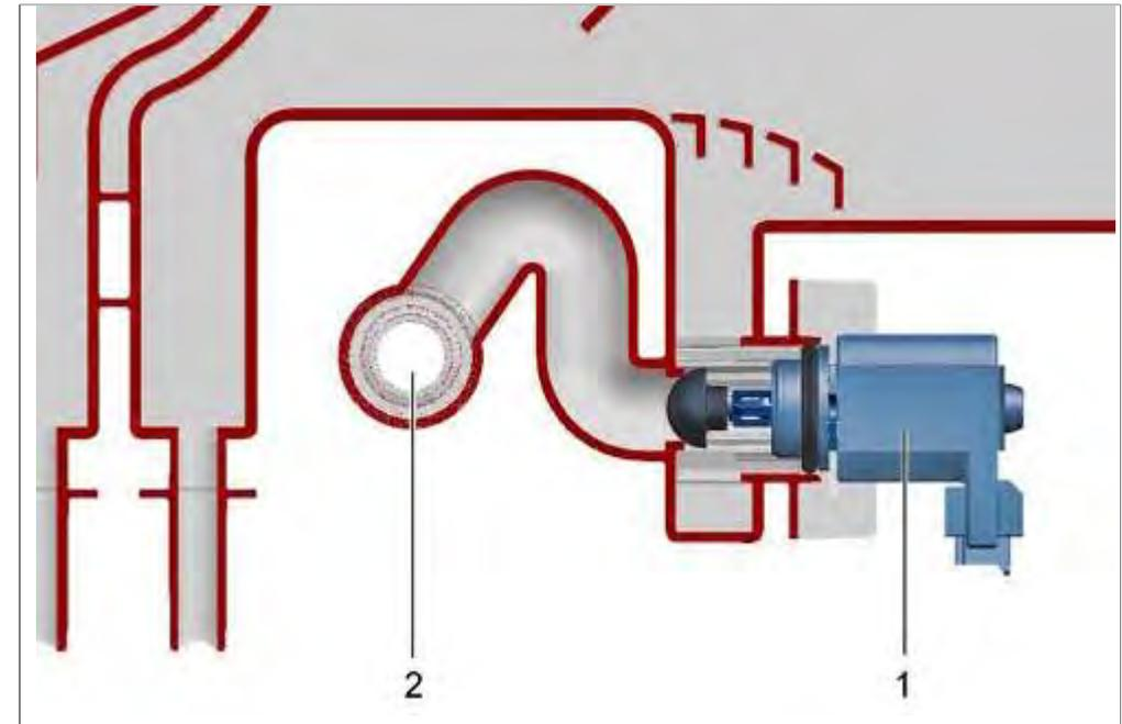
1 Heat exchanger drainage valve
