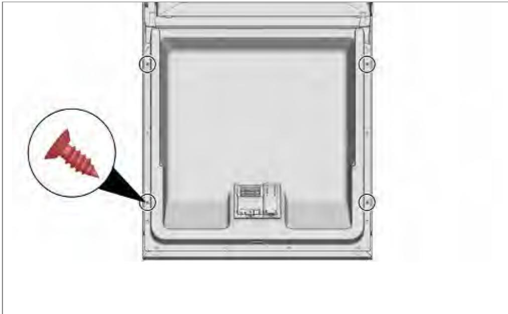
Remove the 2 screws on each side of the inner door.
