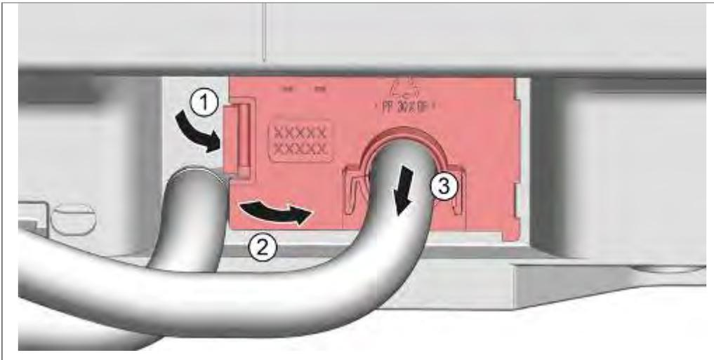
1. Loosen the panel catch mechanism.
