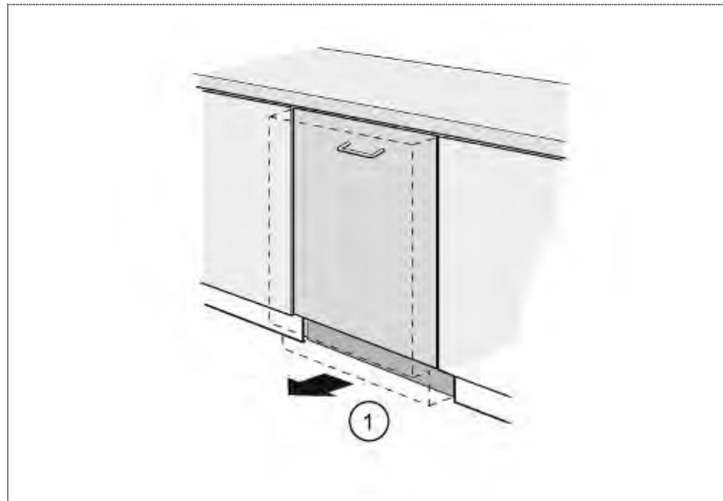
1. Pull appliance out of the installation cavity.
