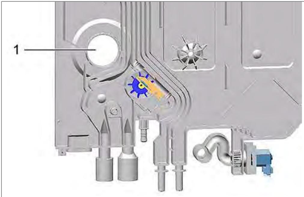
1 Expansion opening in heat exchanger
