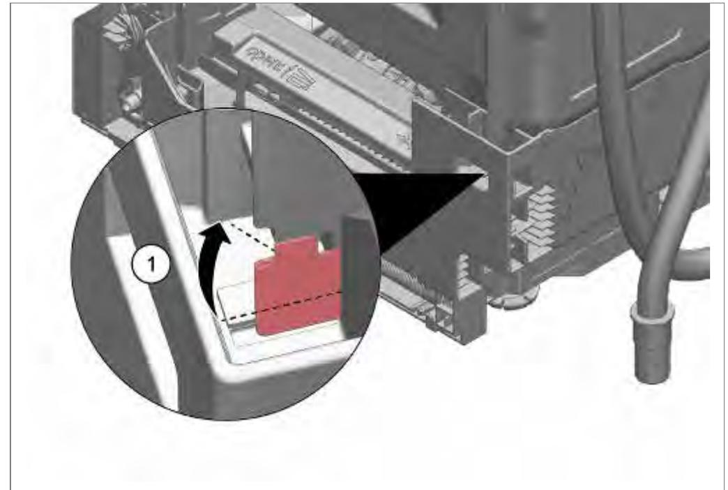
1. Using a screwdriver, bend over sheet-metal brackets.
