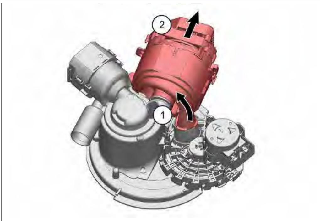
1. Carefully remove/rotate heating pump off the water points hose.
