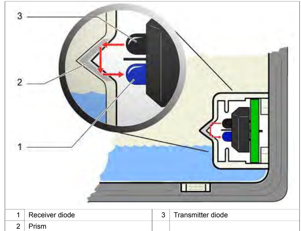
If the dispenser is empty, the light beam in the prism is reflected. The received signal is the same as the transmitted signal.
