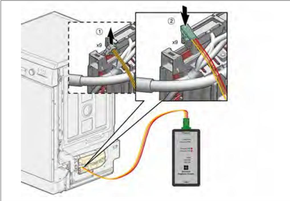
1. The iService connection X9 can be found on the **top** of the module.
