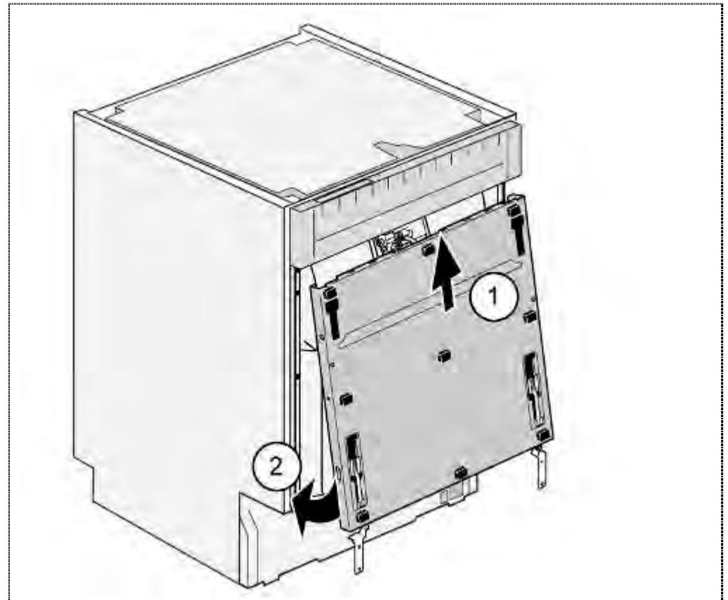
1. Insert outer door from below into the inner door.
