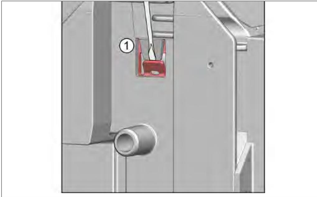
1. Using a screwdriver, bend hinge plate catch mechanism outwards.
