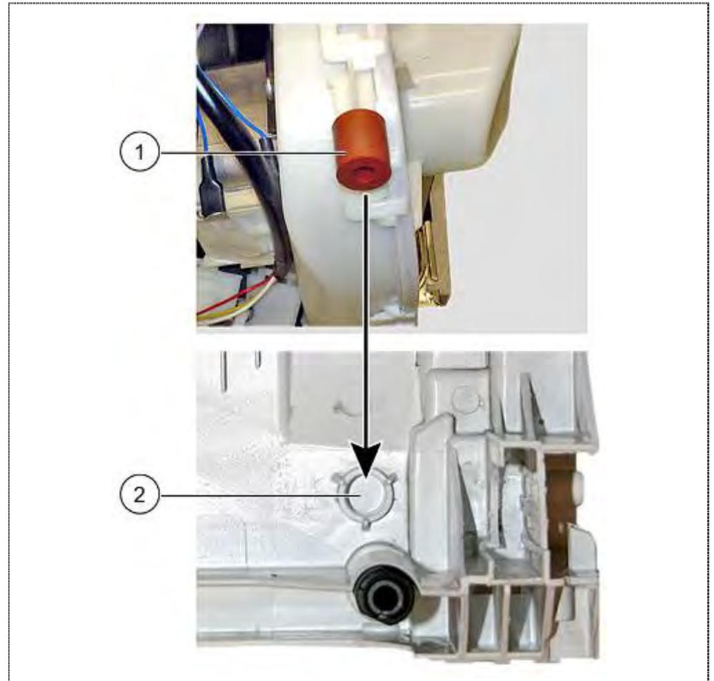
2. Lower housing pin with rubber ring into the base pan.
