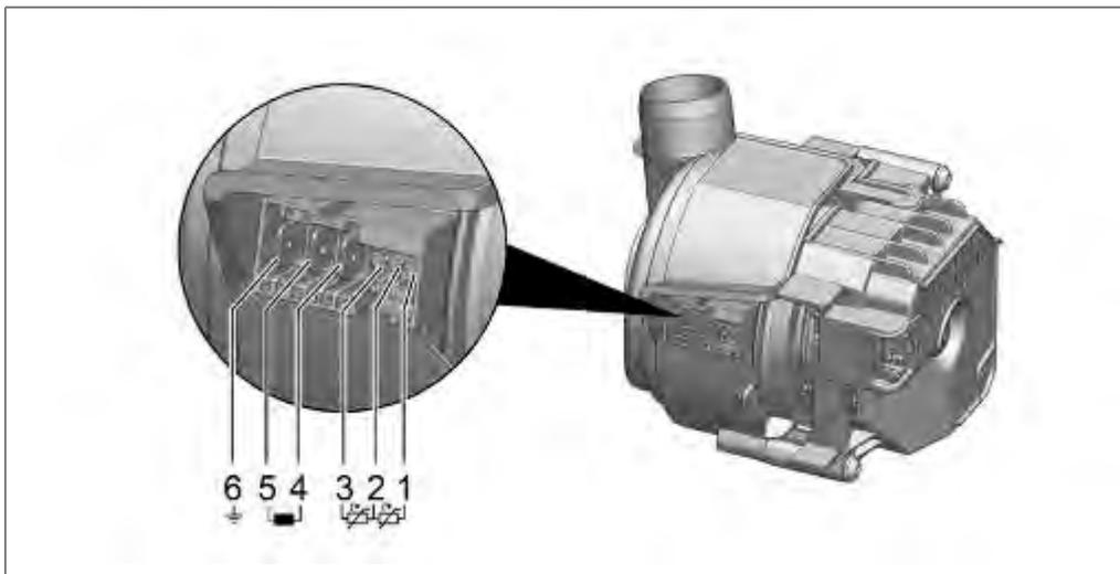
The heater resistance is measured on the heating contacts of the heating pump.
