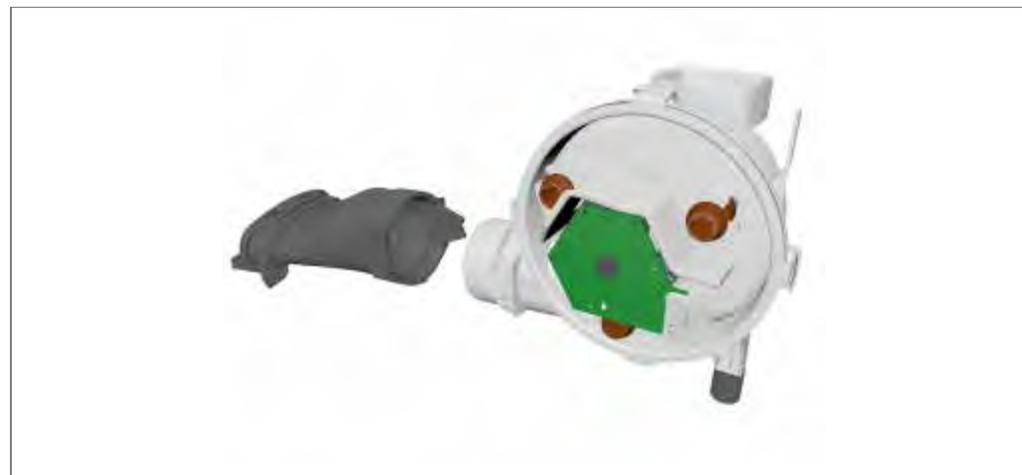
1. Remove fan motor with fan housing from the air channel.
