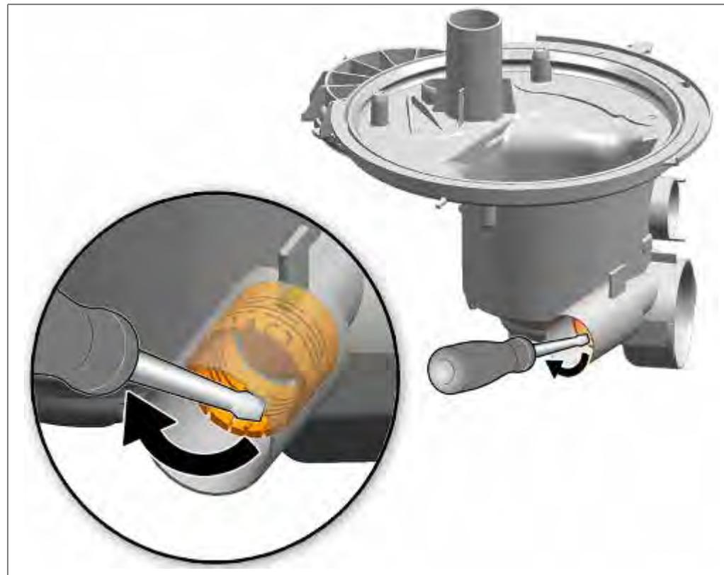
1. Loosen the valve with a screwdriver clockwise and remove it.
