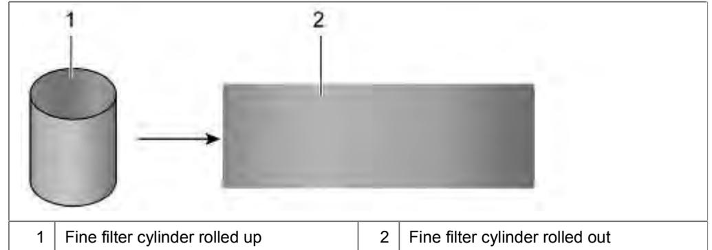
The new fine filter system is based on a corrugated fine filter cylinder. If it is rolled out and smoothed, a 1.5x filter surface can be seen.
