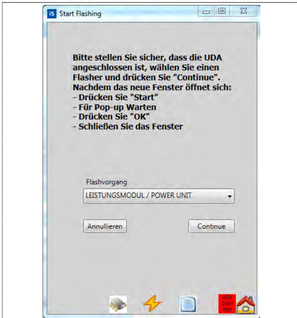
In the field, flash process, the component must be selected, that is to be flashed.
