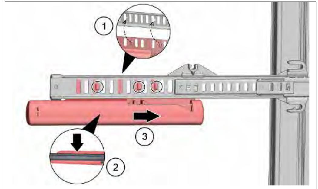
1. Align the soft close mechanism to the special cutouts in the glide.
