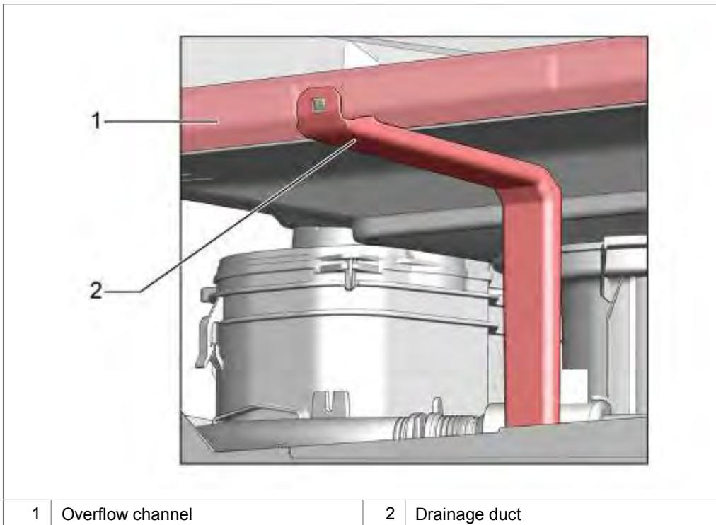
Leakage water is conveyed out of the container via the overflow channel, through the drainage duct and into the base pan.
