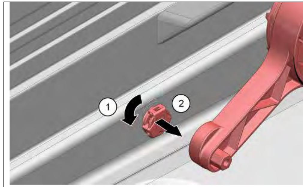
1. Remove cover (optional) on the water inlet in the interior decrease and solve water inlet connection with special tool.
