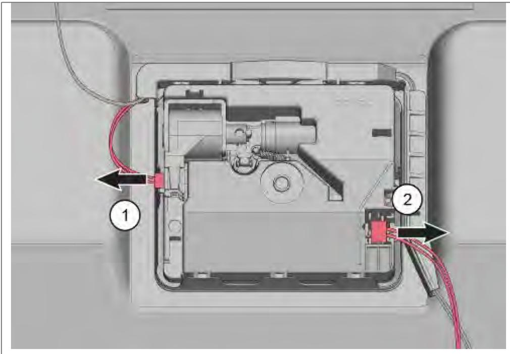
1. Loosen plug-and-socket connection.
