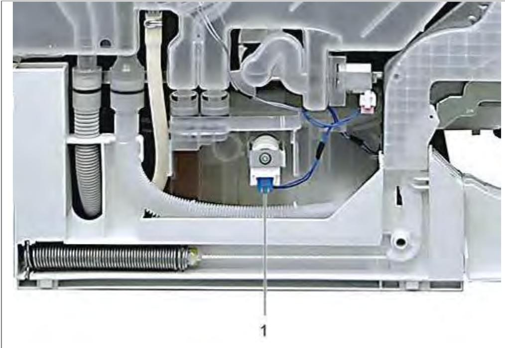
1. Disconnect plug-and-socket connection and measure the resistance.
