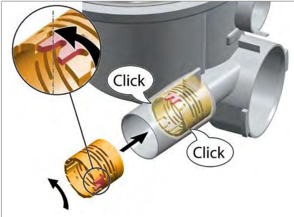
1. Insert the valve in the pump sump.
