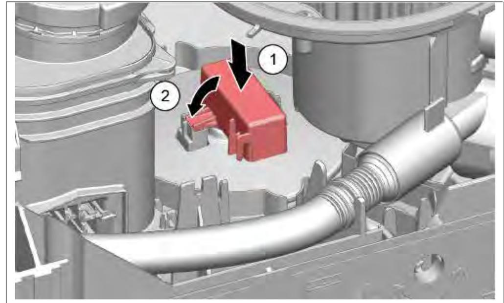
1. Press float switch into the catch mechanism of the base plate.
