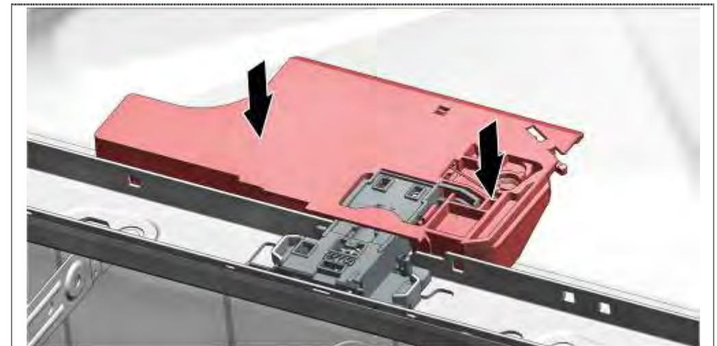
1. Door open module just snaps into place from above.
