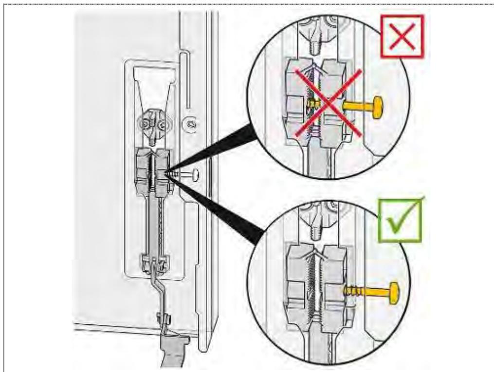
Check the locking screws. The guide part cannot be positioned securely unless the gap between the sliding elements is free. The screws must be unscrewed far enough.
