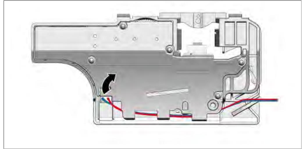
Remove doorway module. Disconnect cable connection.
