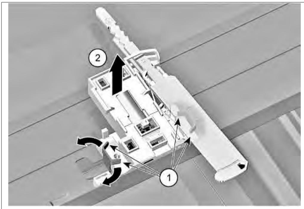
1. Straighten metal brackets on right and left of the door lock.
