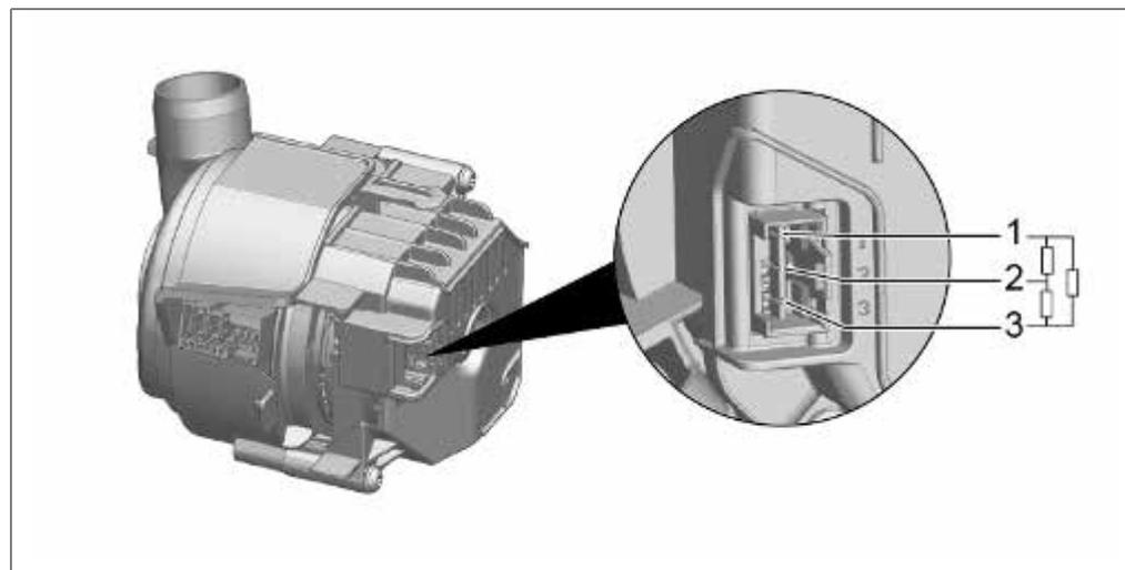
Measure winding resistance on the winding contacts of the heating pump.
