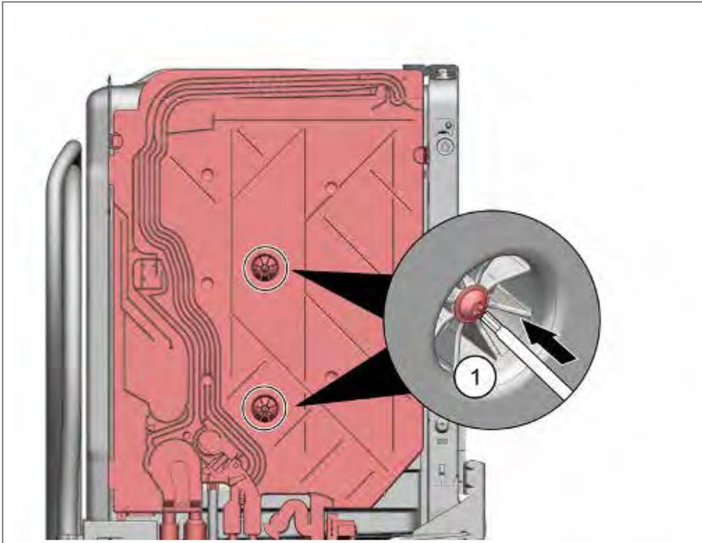
1. Screw heat exchanger with the container.
