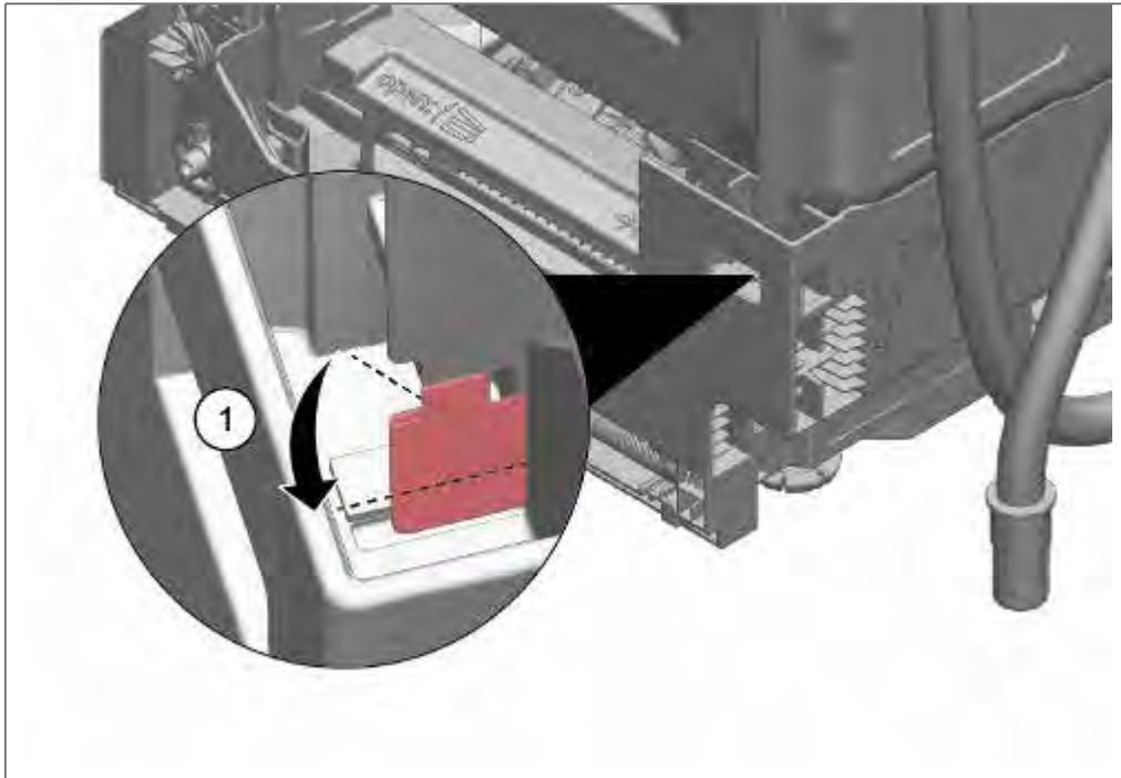
1. Using a screwdriver, straighten sheet-metal brackets.
