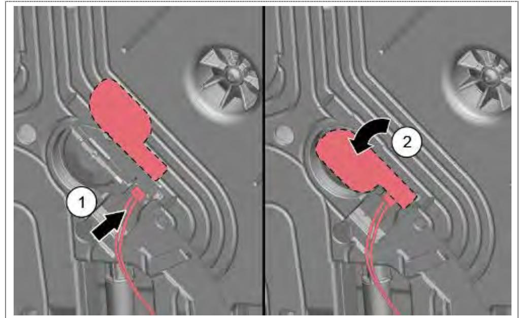
1. Connect connector to the impeller PCB.
