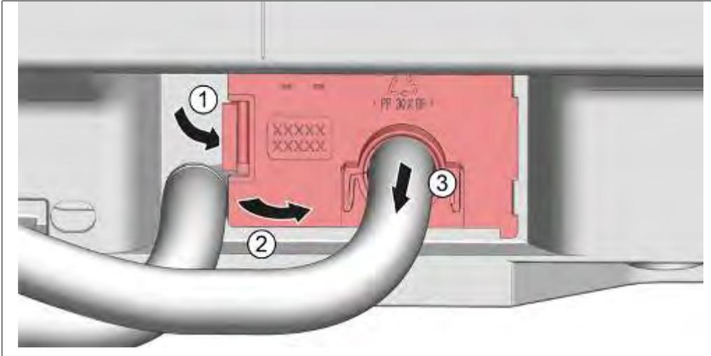
1. Loosen the panel catch mechanism.
