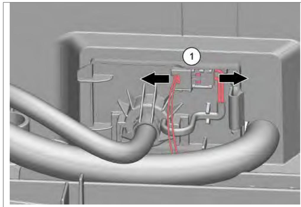
1. . Disconnect plug-and-socket connection.
