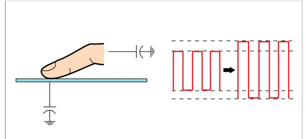
The capacity depends on the print and the strength of the materials of the control panel. To ensure a safe response of buttons, each control module must be adapted to the aperture. This is done via the software with specific parameters.
