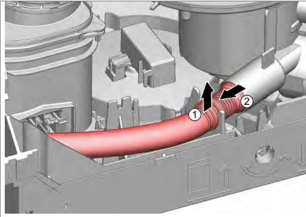
1. Press flexible drainage hose upwards out of the fixing.
