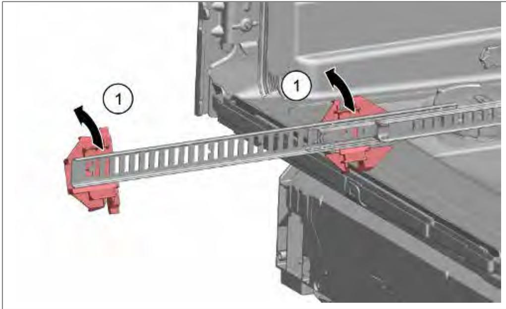
1. Snap the rack holder off the glides with an outward motion.
