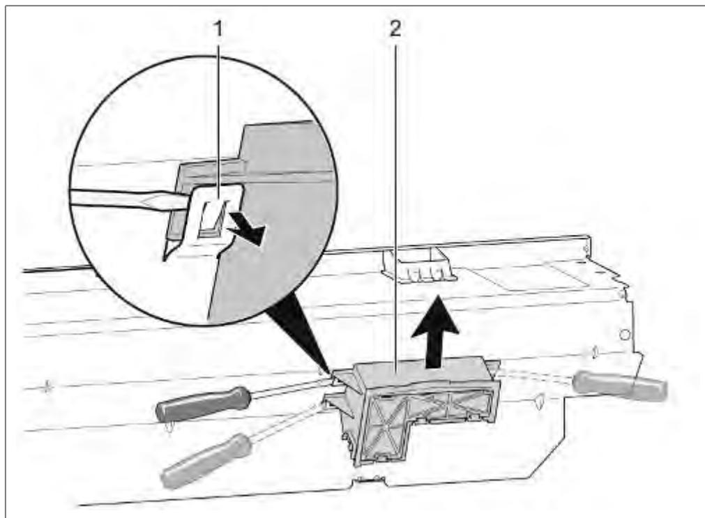
Bend the latches (1) back before installation.
