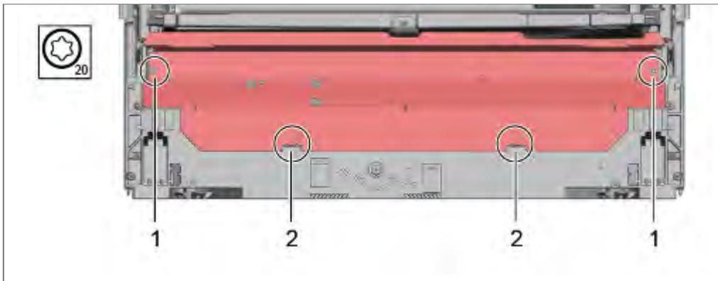
1. Loosen base plate by unscrewing the Torx screws.
