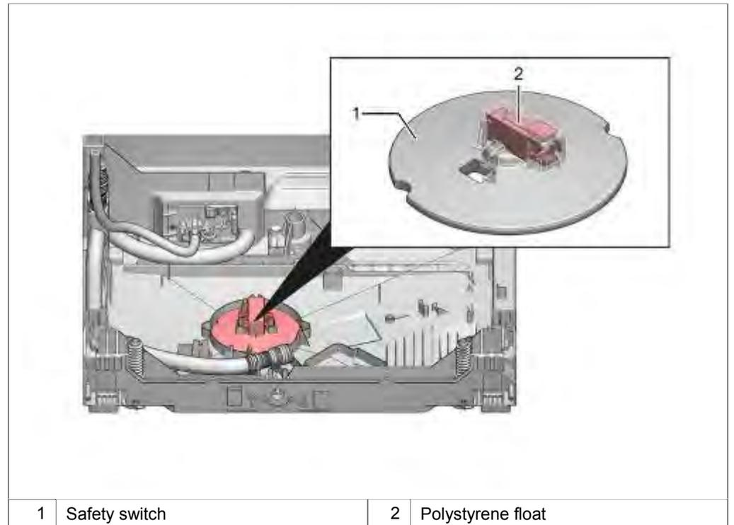
The safety switch is mechanically connected to the polystyrene float.
