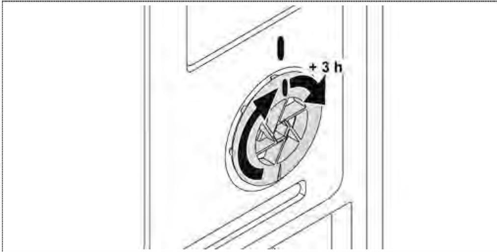
1. To prevent leakage, around the value + 3 hours (1/4 revolution) continue to tighten.
