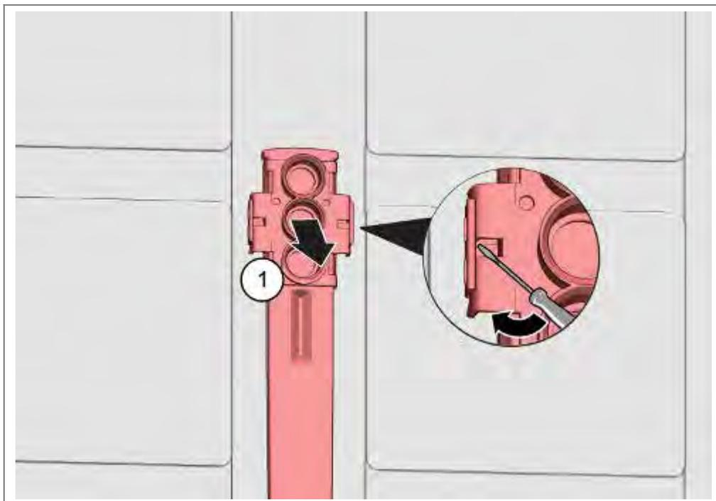
1. Release catches in the area of coupling point.
