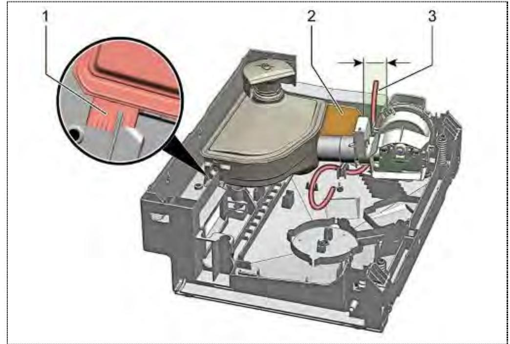
1. Ensure that the zeolite container is in the guide.
