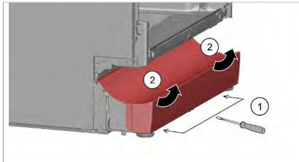
The underside of the base panel is secured with 2 catches.
