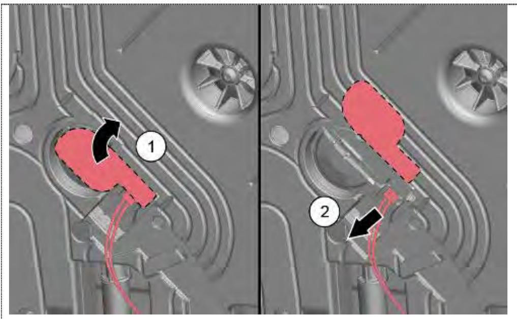
1. Bend out the guard cover of the impeller wheel counter.
