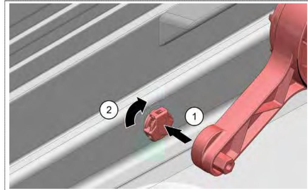
1. Insert Water inlet connection, tighten it and push cap (optional) onto the water inlet connection
