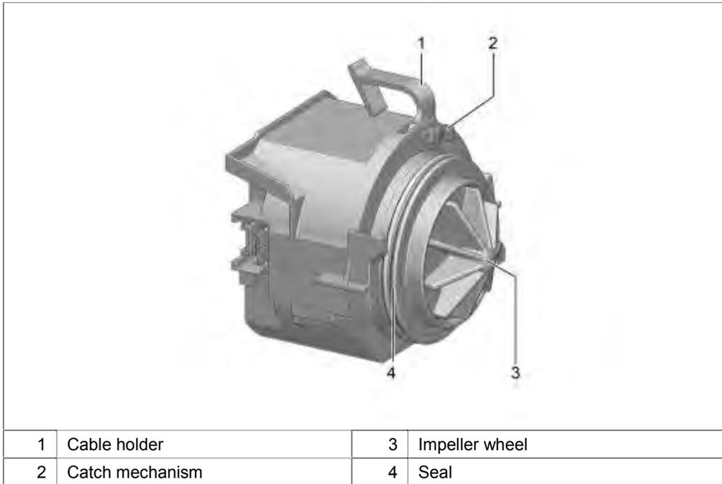
The water is drawn in via the water outlet opening of the pump sump. The impeller wheel pumps the water through the non-return valve into the drainage hose.
