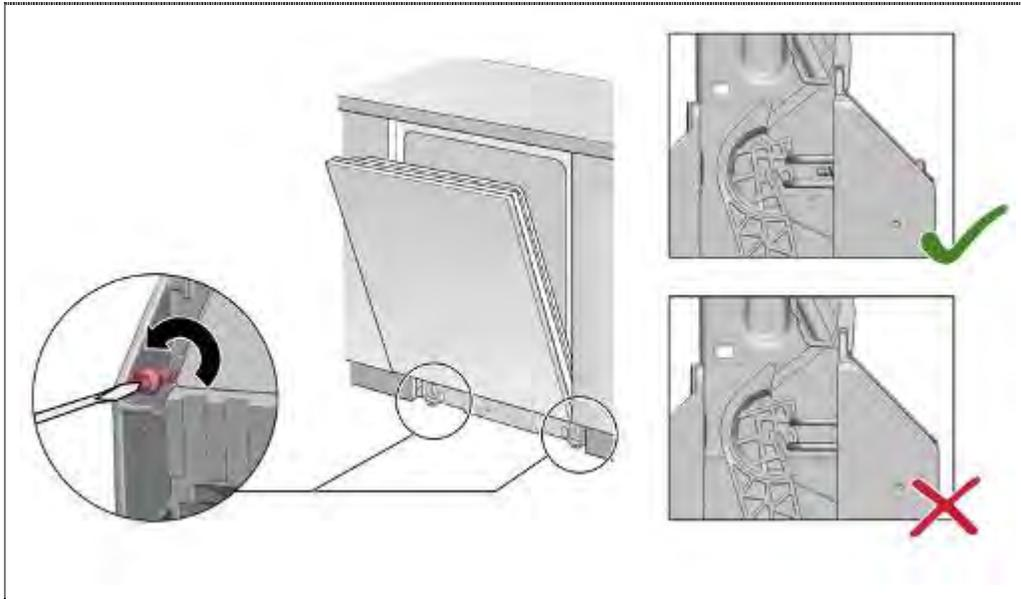
Loosen the adjustment screws.
