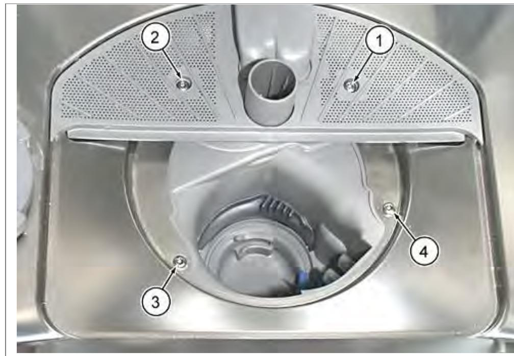
Loosen 4 screws (1. to 4.) in the interior container and remove pump sump downwards.
