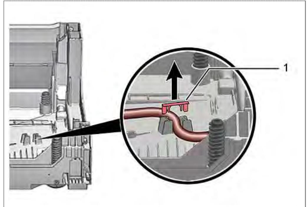
1. For devices with fleet storage is to remove the retaining clip (1) of the tube gently.
