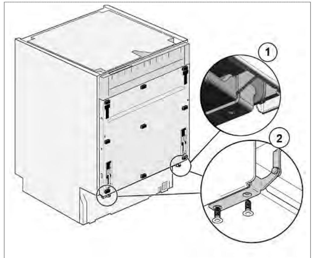
1. Mount the joint on the hinge side plate and screw in from below.
