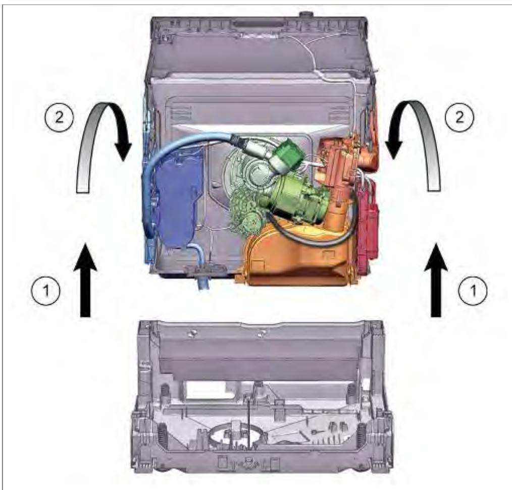
1. Carefully lift rinsing tank upwards.
