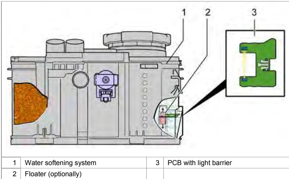
The PCB for the low salt indicator is attached with clips to the right side of the water softening system (front side of appliance).
