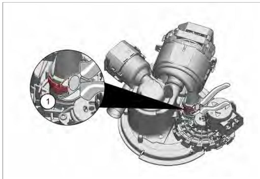
1. Using side cutters, loosen the hose clamp on the water points connection.
