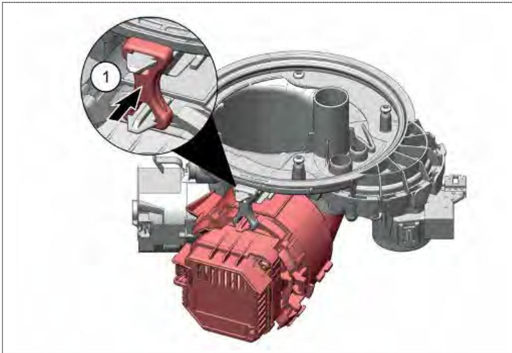
1. Attach rubber mount between the pump unit and pump sump well
