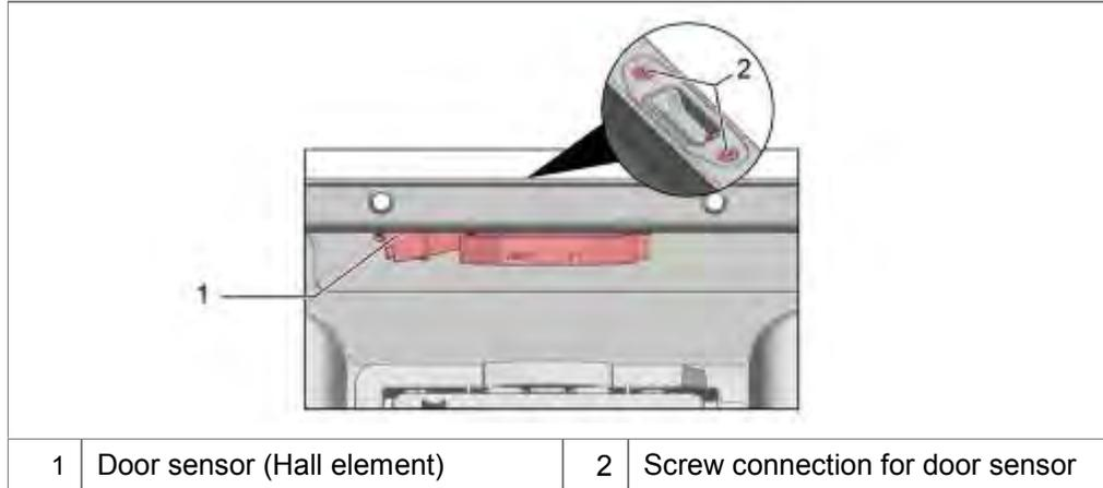
The door sensor is situated in the centre at the top of the inner door.
