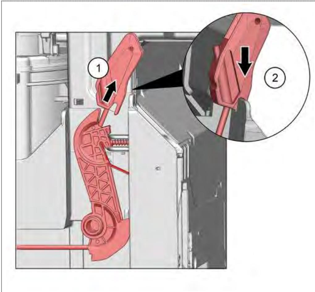
1. Pull rope holder upwards.
