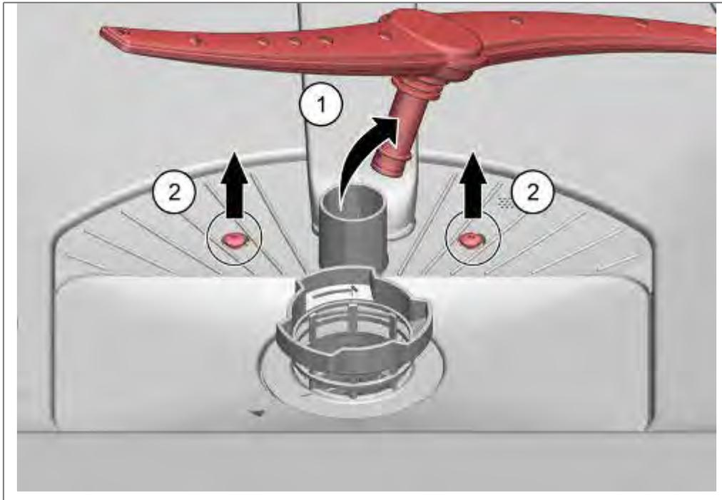
1. Pull off the lower spray arm with a slight jolt up the feed tube.
