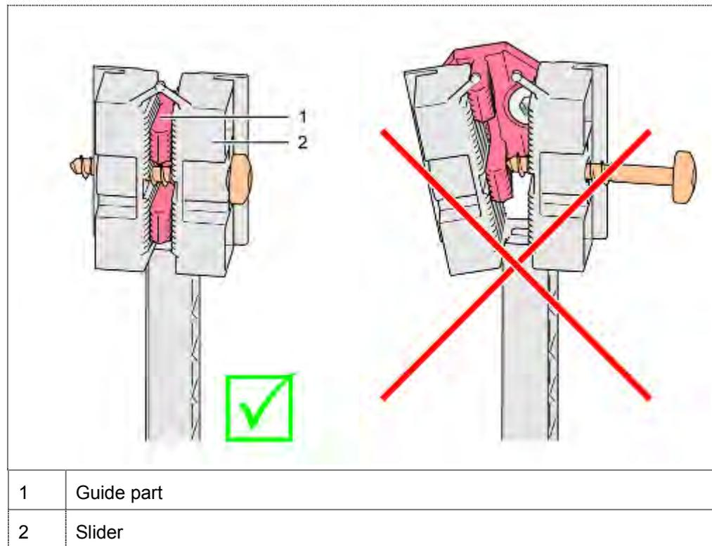
The guide part has to be positioned in such a way in the sliding elements, that the locking screw is in the centric recess.
