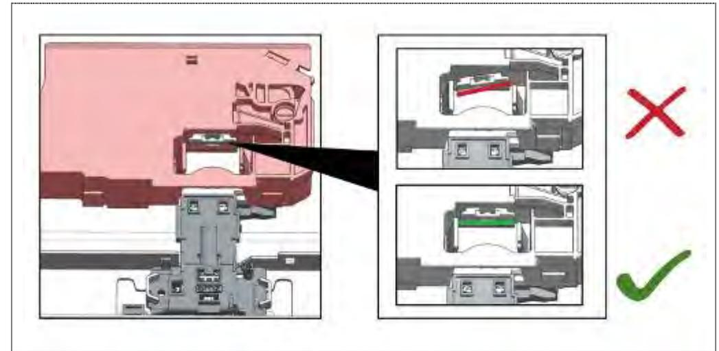
1. Align the sensor plate before installing.
