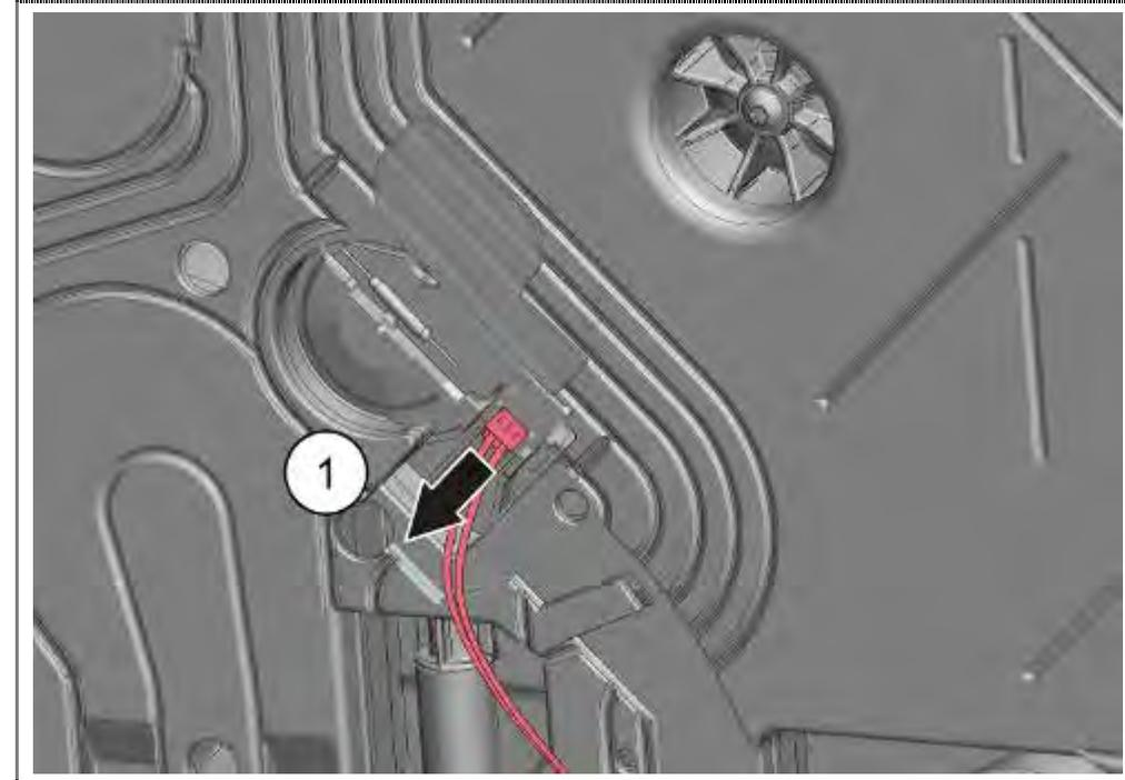
1. Loosen plug-and-socket connection
