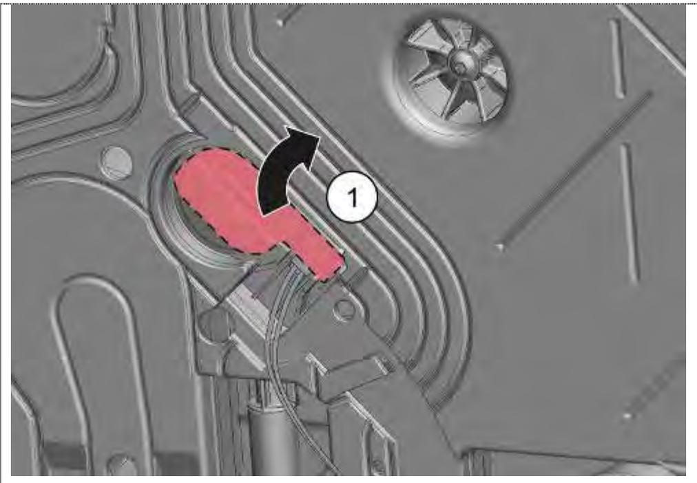
1. Carefully bend out the plastic flap on the heat exchanger / water inlet.
