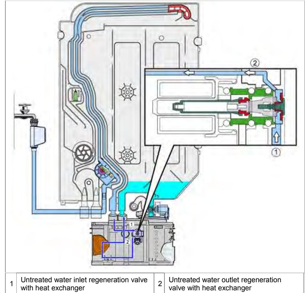
If the regeneration valve is actuated, the water flows into the salt dispenser and is enriched with salt.
