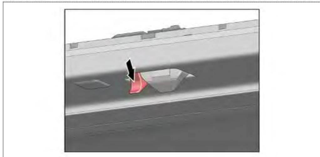
1. Press the lever to „closed“ position.
