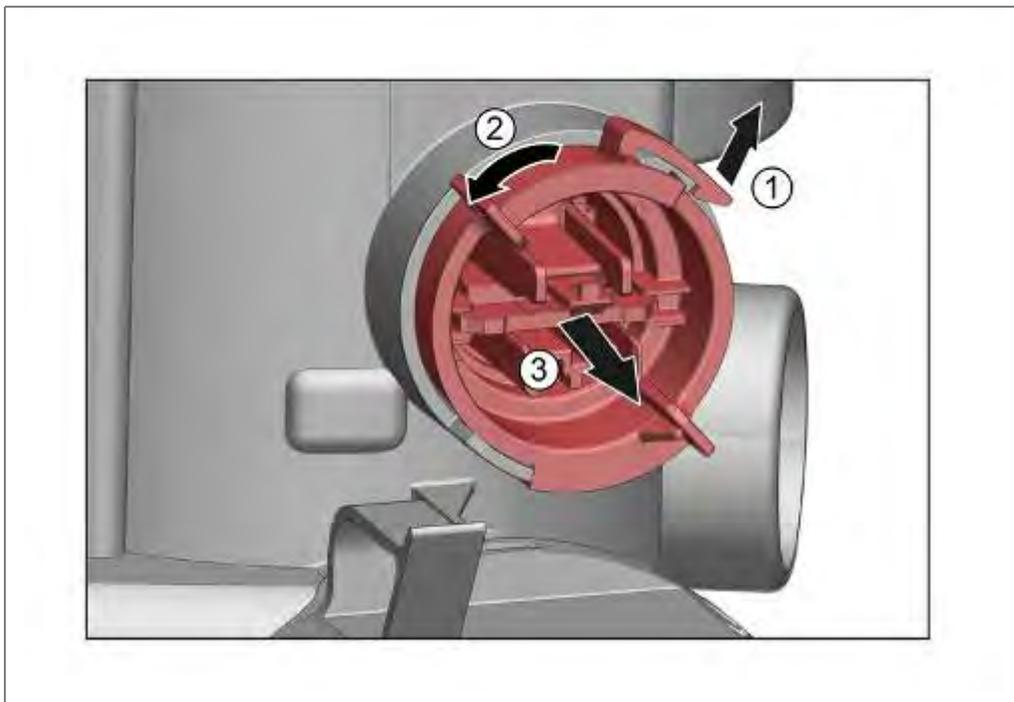
1. Loosen catch mechanism.
