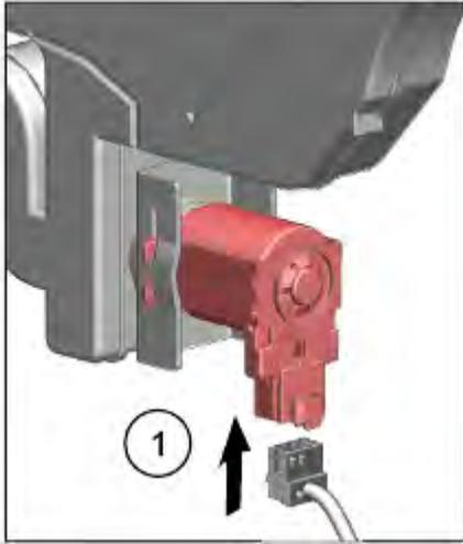
1. Establish plug connection on the drain valve again.
