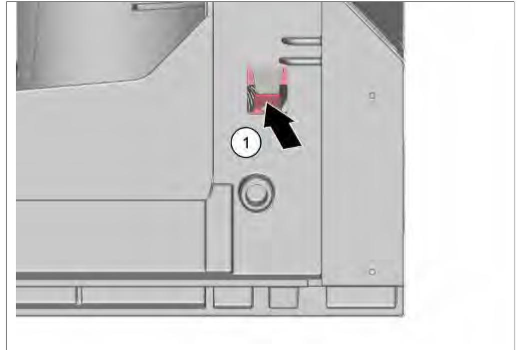
1. Using a screwdriver, detach hinge plates at the front side from the top of the catch mechanism. To do this, bend in the hinge plate catch mechanism.
