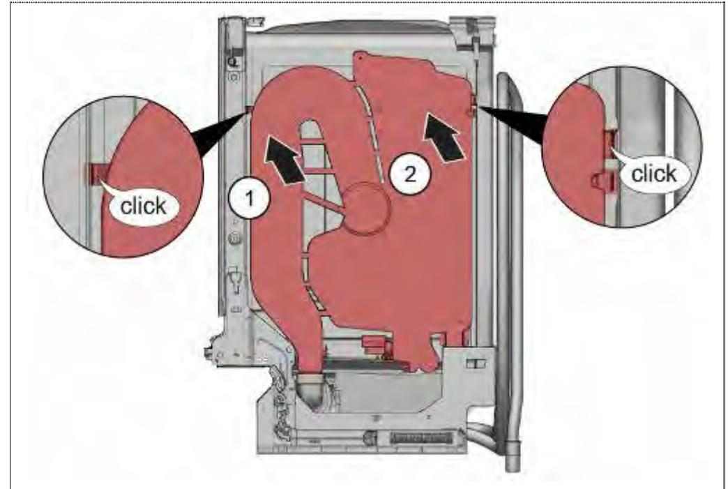
1. Insert the liquor reservoir / duct to the catch.
