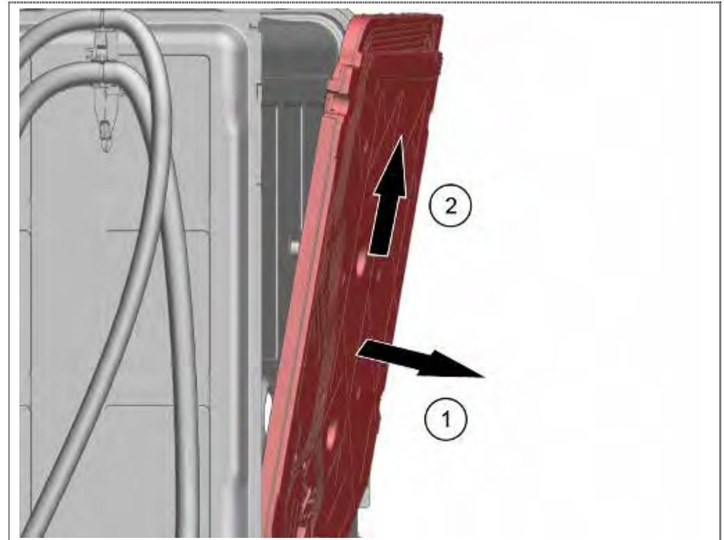
1. Carefully separate heat exchanger above the container.
