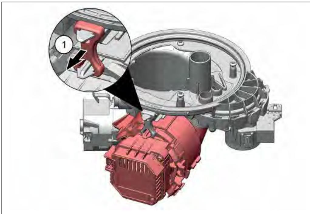
1. Detach rubber holder from between pump unit and pump sump.
