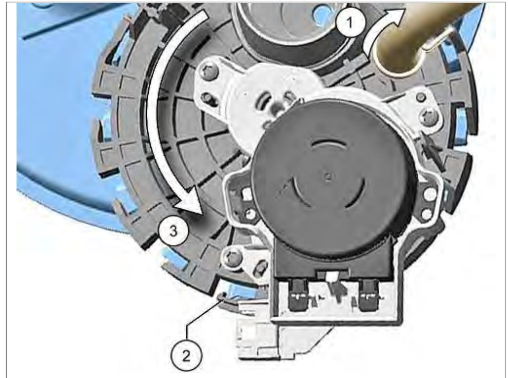
1. Remove the hose for water storage tank (optionally)
