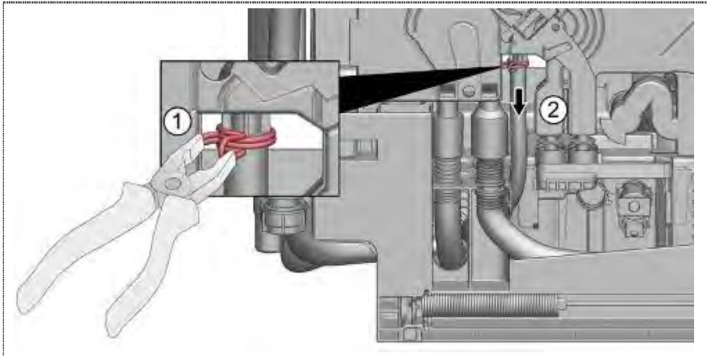
1. Loosen hose clamp on the water supply
