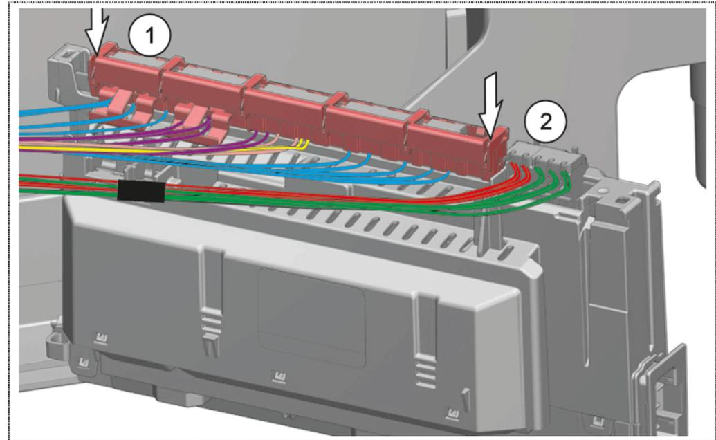
1. Insert coding frame into the guide.
