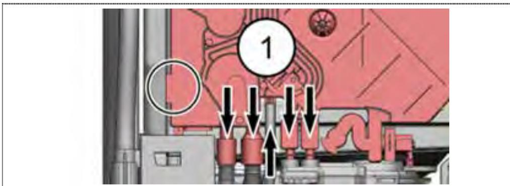
1. Ensure that the connection is faultless without crushing the terminals on the heat exchanger.
