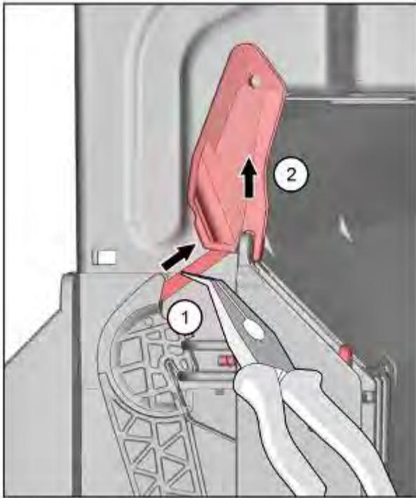
1. Grip tension cord with flat-nosed pliers.
