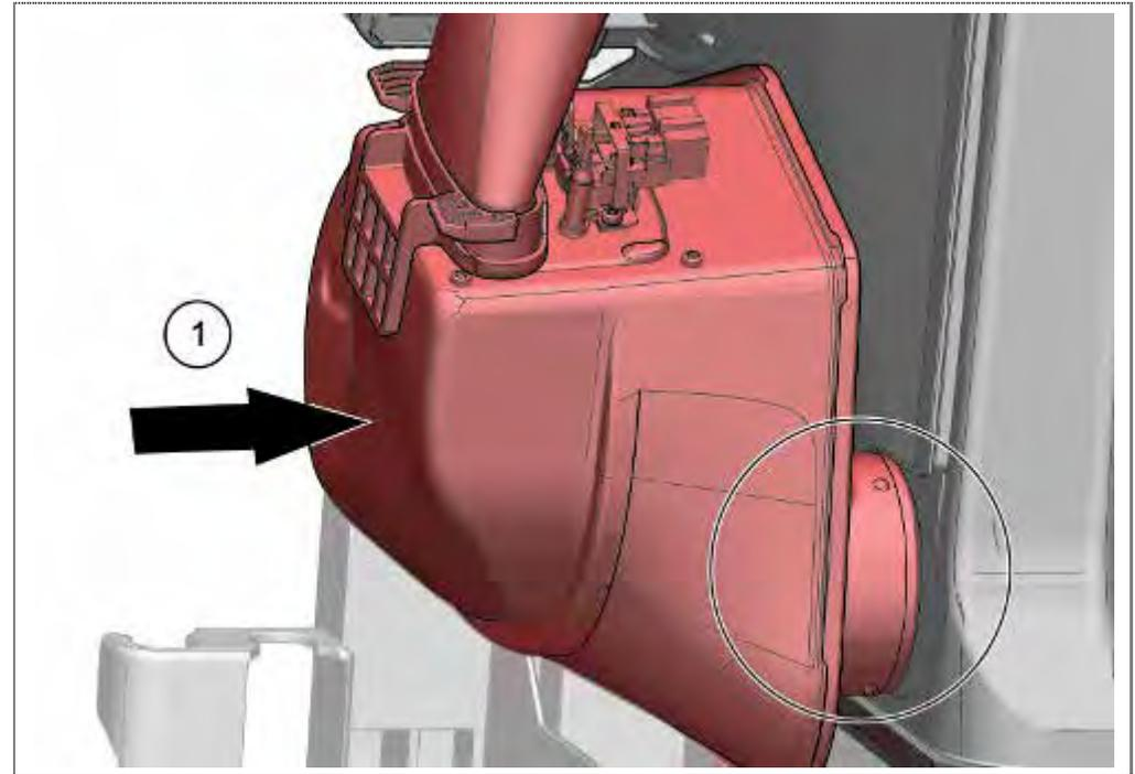
1. Insert zeolite container gently into the opening of the tub.
