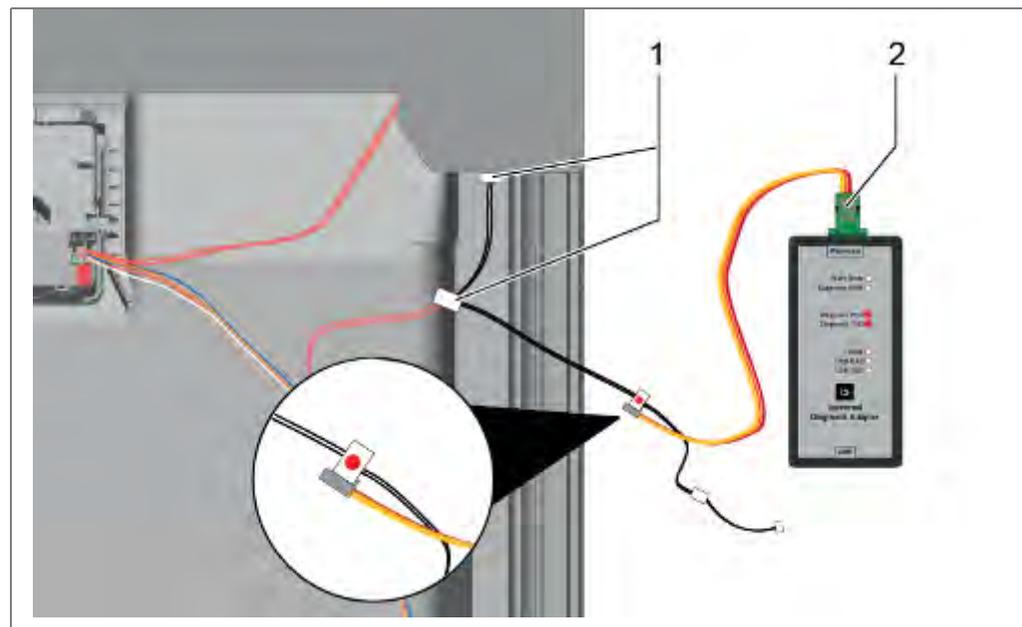
3. Connect the Y cable to the control module. Depending on the model, the 3 wire or 4 wire connection of the adaptor (341248) should be used. There will always be two connectors that are not used.
